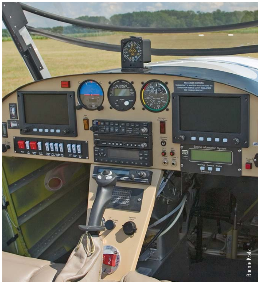
Above, the instrument panel of an amateur-built Zenith 601 XL. Below, the panel from the AMD 601XL S-LSA. The 601 XL's panel is designed to accommodate a wide variety of instruments including all of the latest digital instruments and avionics.
