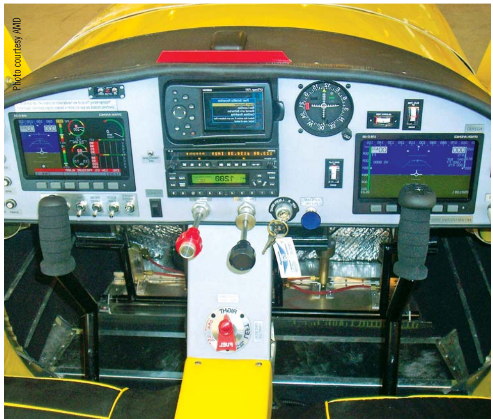
Above, the instrument panel of an amateur-built Zenith 601 XL. Below, the panel from the AMD 601XL S-LSA. The 601 XL's panel is designed to accommodate a wide variety of instruments including all of the latest digital instruments and avionics.
