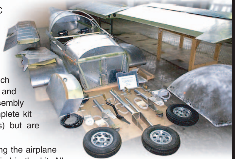
A partially assembled Zodiac airframe
