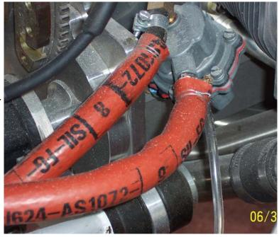
Attach the 3/16 clear plastic hose to the small nipple on the fuel pump and route it so that any discharge will be away from the hot exhaust system components.
