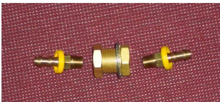
Locate a good place for the fitting to be installed in the firewall. Locate it to the right of the nose leg channel in a spot where it will not interfere with the throttle cable. Drill a 3/4 inch hole in the firewall at the chosen location.
