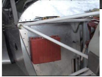
It is recommended that the battery be placed as far left as possible so as to make space for the oil recovery kit and the cabin heat option. Plan the right side of the firewall to be taken by the air box.
