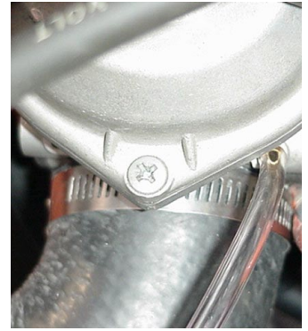
Vent hose CH-4 Connect with 1/4" plastic hose the nipple on the right side of carb to nipple on the air box
