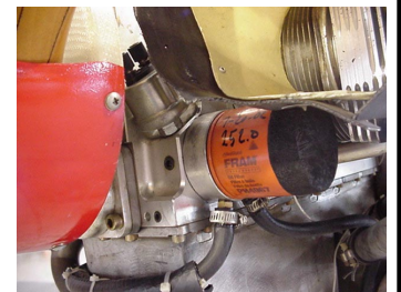
Screw the adapter between the engine and the oil filter.
