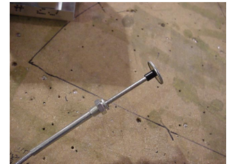
Cable pulled out "CARB HEAT ON"
