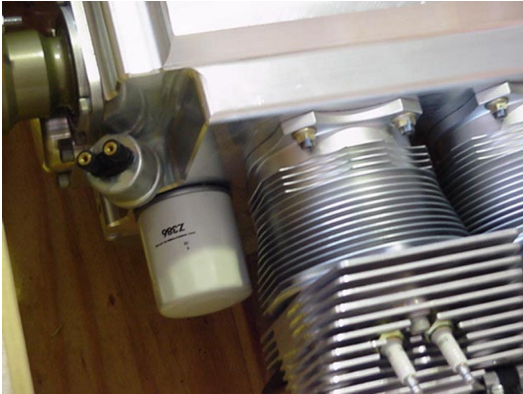
Location of the oil filter in front of cylinder #2
