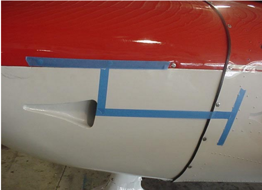
Location of scoop on left side of cowl.
