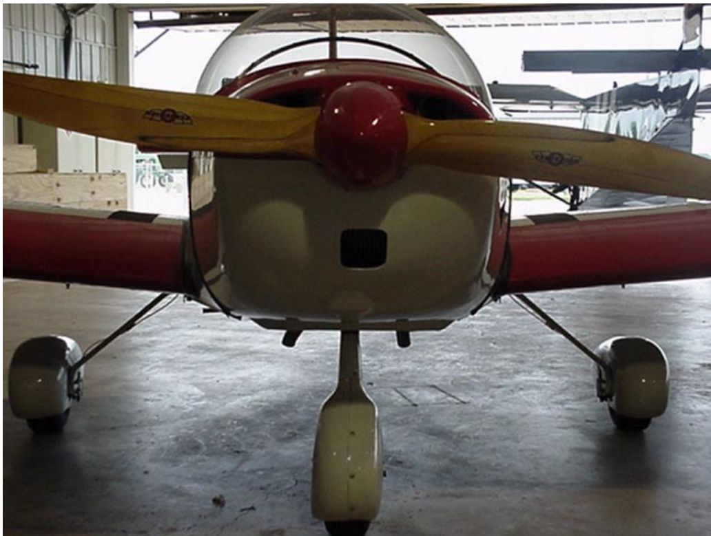
Front view showing the muffler outlets below the fuselage.
