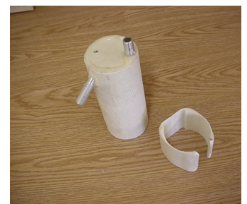
Fiberglass part. The clip is riveted to the firewall.
