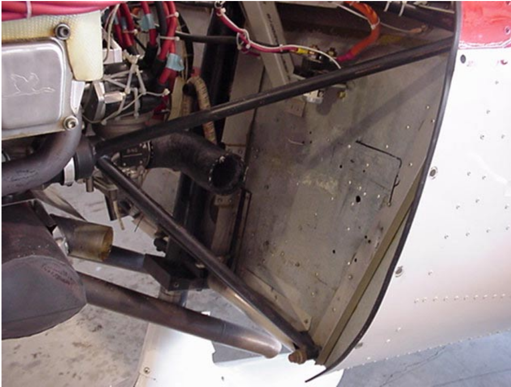
Space on firewall to mount the air box
