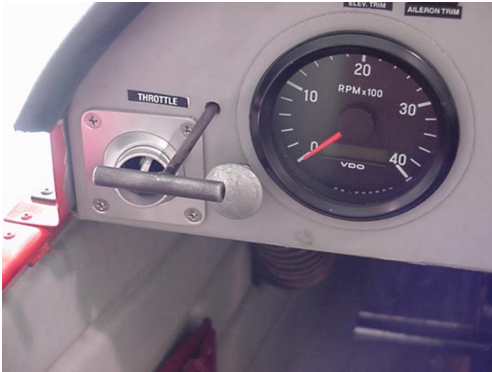
Dual throttle, detail of left side.
