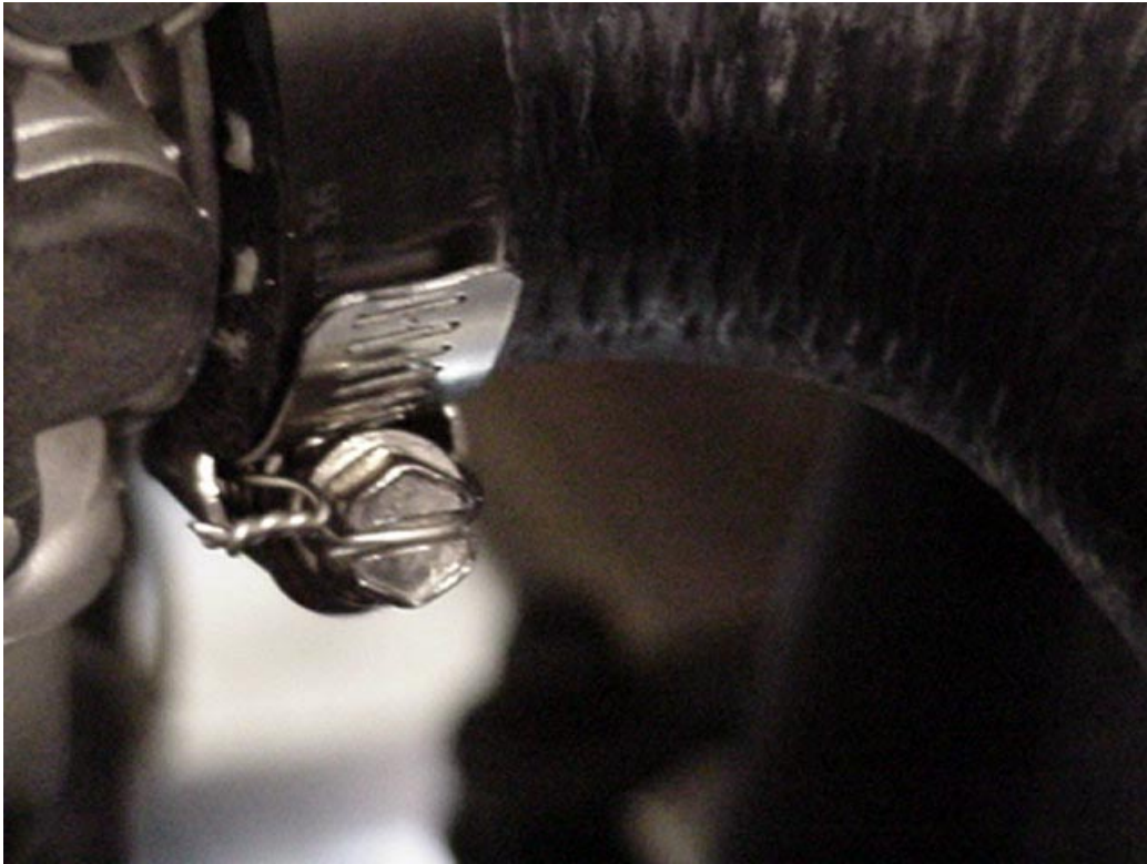
Safety wire on all hose clamps
