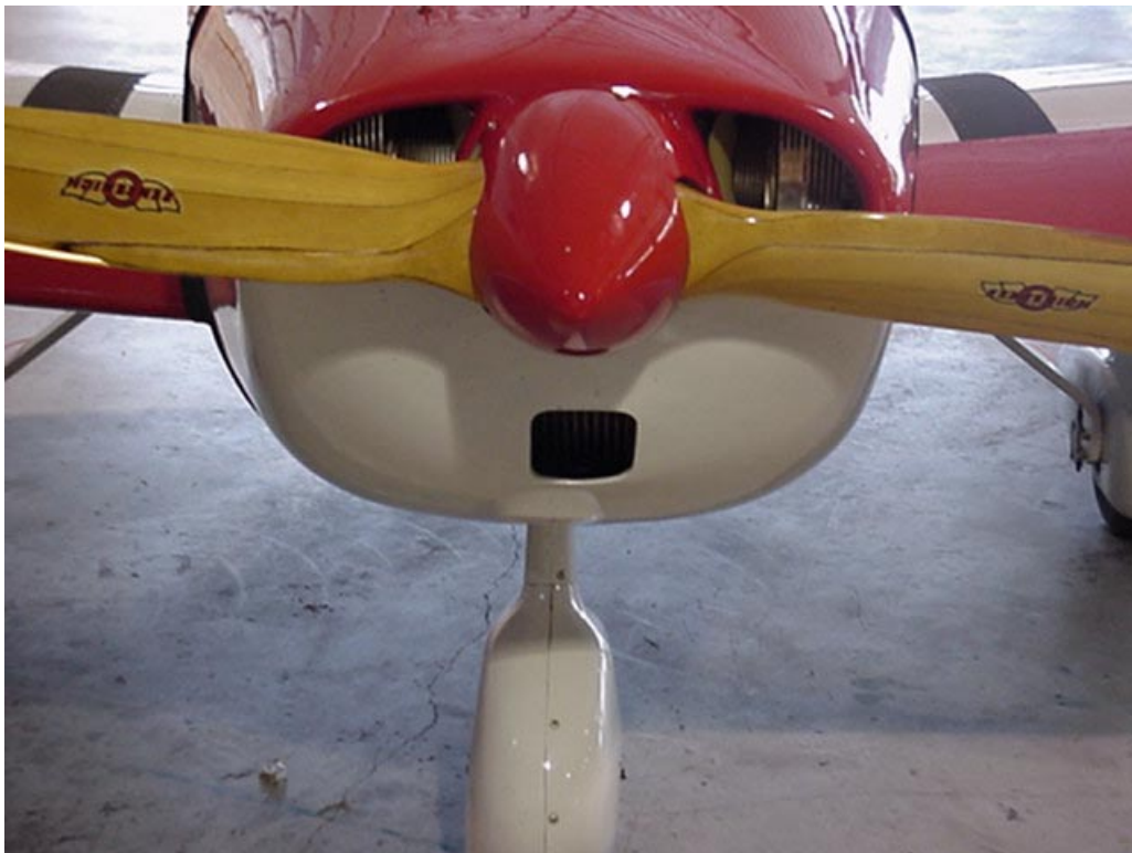
Trim the baffle to fit the cowl.
