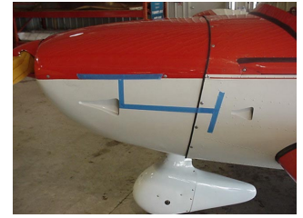
Location of scoop on left side of cowl.
