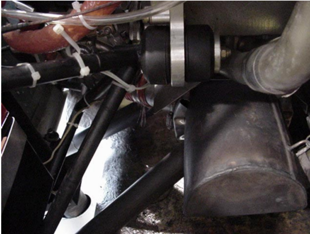
Muffler installed with bottom cowl in place.
