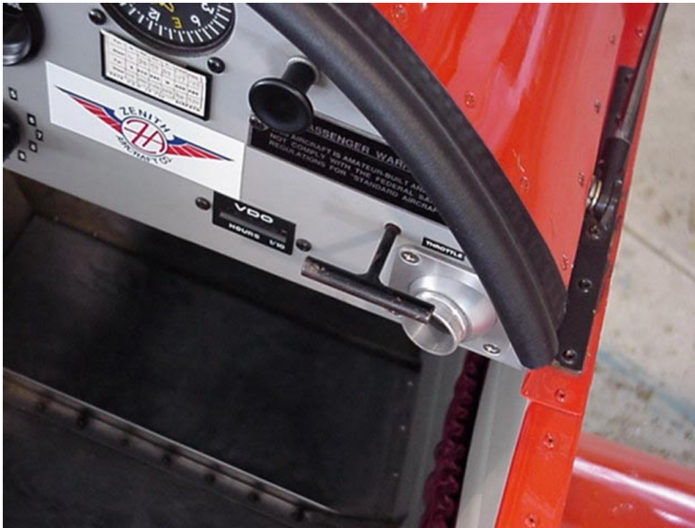
Pulled back idle, the stop is on the carburetor
