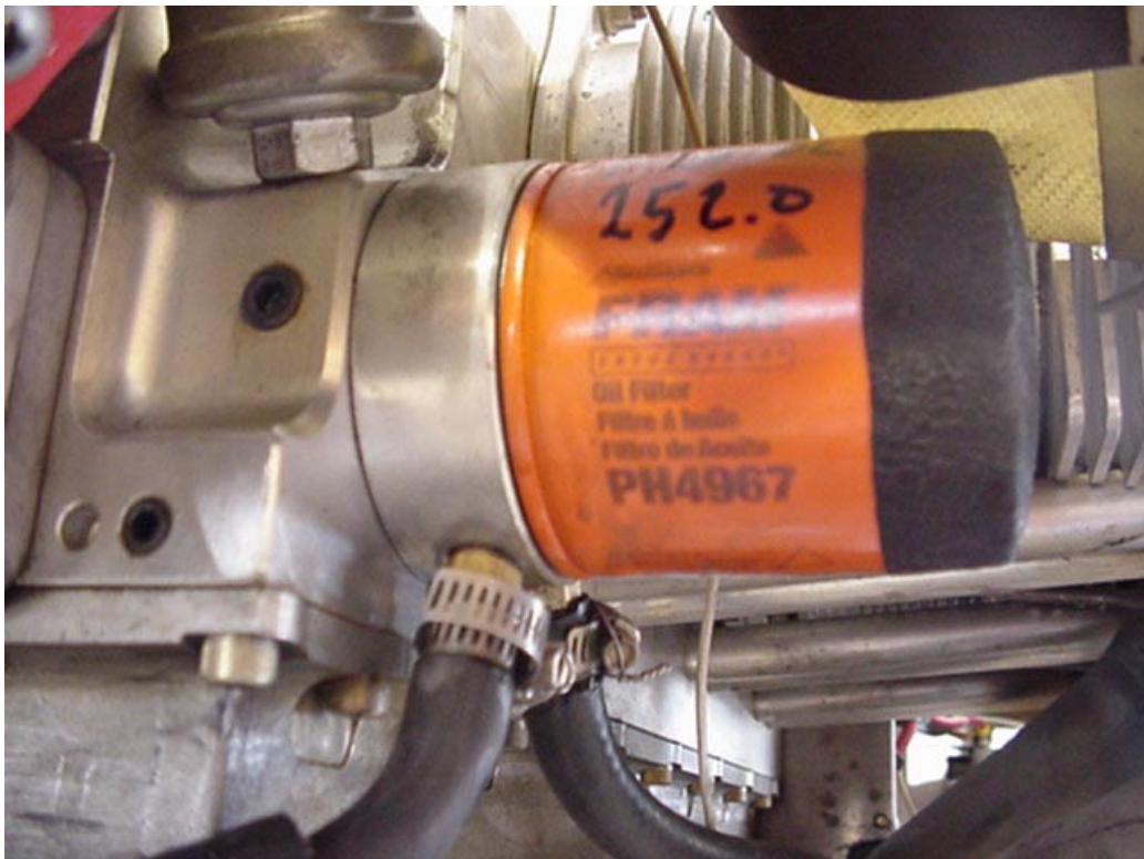
Suggestion: mark the date and hours on the oil filter
