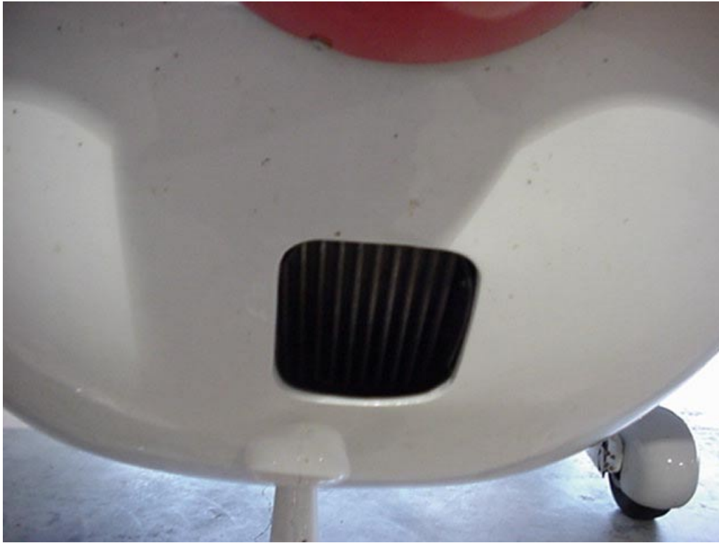
Cutout in the bottom cowl in line with the oil cooler.
