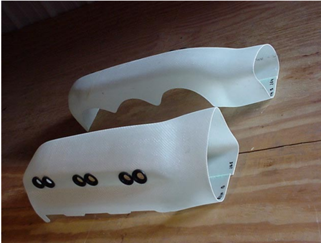
Ram Air Ducts – Tractor
