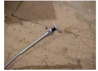
Cable pushed in "CARB HEAT OFF"
