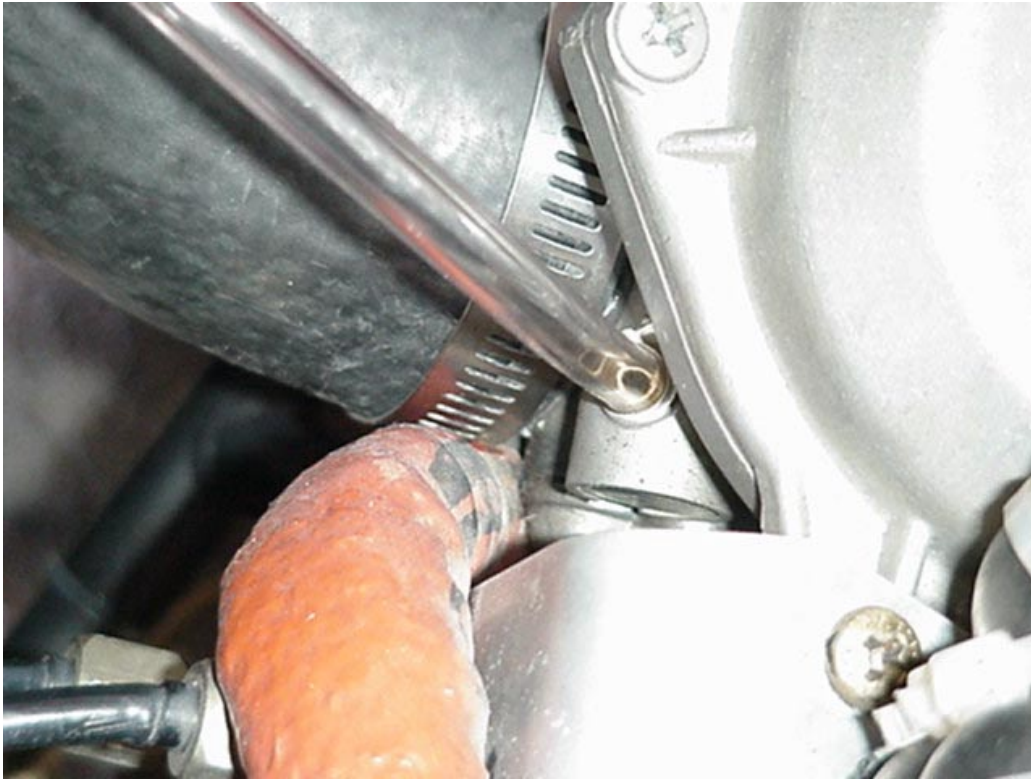
Detail of 1/4" hose on right side of carb.
