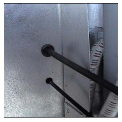
Mount the cable in the panel and route the cable forward and down and through the firewall grommet. Make sure to avoid interference with other wires and structures.
