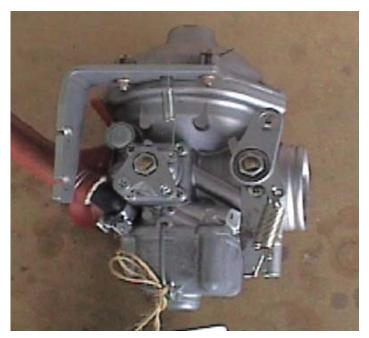
2. With the carb on the bench, cover all openings of the carb with tape to prevent any debris from entering the interior of the carb. Remove the throttle bracket from the carb
