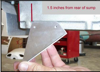
2. Drill through the outside fin using the pre-drilled holes in the Aluminum bracket as your drilling jig.
