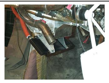
5. Position the radiator so that it is centered in the cooling air inlet. Make sure there is clearance of around the cooler so that the radiator will not contact the cowl. Most installations will have about 3/4 inch clearance between cowl and radiator at the bottom. Position the radiator so that clearance is no more than 3/4 inch. When happy with the position of the cooler, screw the cooler onto the bracket with self tapping screws or firmly clamp in place to maintain the correct position
