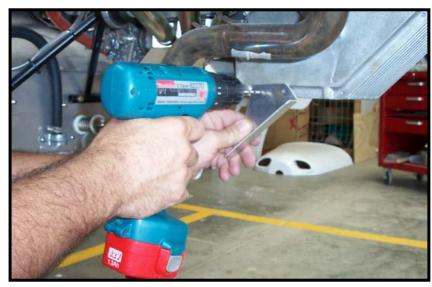
3. Rivet into position using two 3/16 blind rivets on each bracket.
