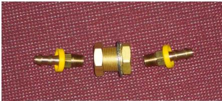
Locate a good place for the fitting to be installed in the firewall. Locate it to the right of the nose leg channel in a spot where it will not interfere with the throttle cable. Drill a 3/4 inch hole in the firewall at the chosen location.
