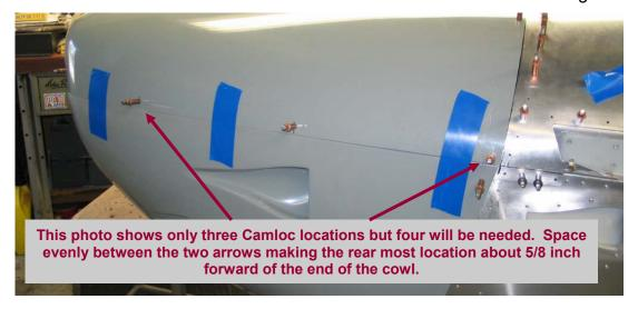
Finally Evenly space the two Camlocs on the top rear of the upper cowl. Drill to 1/8 and install clecos to hold the cowls in place.
