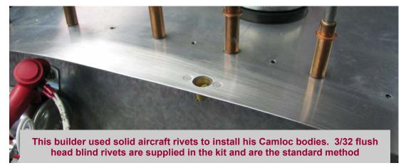
Drill a 1/4 inch hole in the upper cowl for the Camloc insert. Make a small notch in one side of the hole to allow the pin to fit through. On the sides of the cowl the Camloc bodies are installed on the back side of the joggle joint and #6 Camloc inserts are used. At the top rear the bodies are riveted to the under side of the fuselage skin and #2 Camolc inserts are used.
