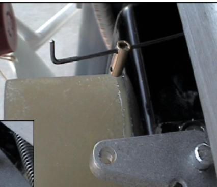
7.- Install the brass pin into the lever. Solder the brass pin to the end of the carb heat cable.
