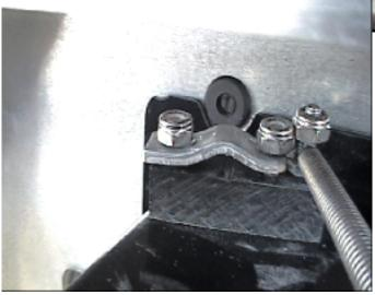
2.- Mark and drill a hole through the firewall in line with the cable attachment point on the air box. You will need to cut out the air box flange where the cable will run through. (Place a rubber grommet) 3.- Run the carb heat cable through the firewall. Cut the cable housing to length.
