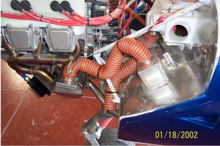
the firewall.. This photo shows a Jabiru J series where the box is on the left. Final position is left to the kit builder. Place the stainless steel side of the box through a 2" hole drilled through the firewall.
