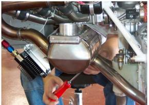
Slide the muff back in place on the muffler and check for clearance between the manifold heat shield and the muff and the exhaust manifold pipes and the muff. Adjust further if necessary by bending the flanges or notching around the pipes.
