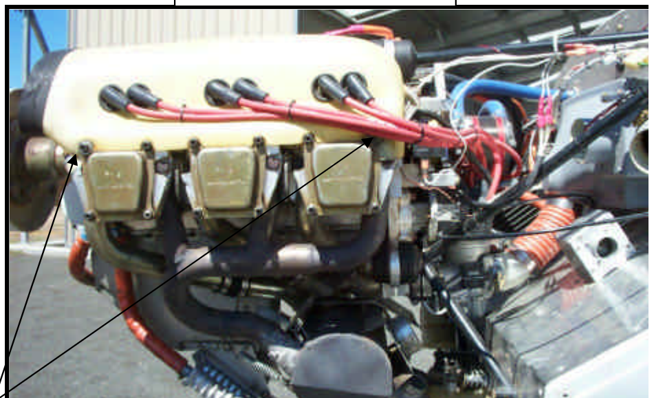
Front & Rear tappet cover Cap Screws used for securing Ram Air Cooling Ducts.
