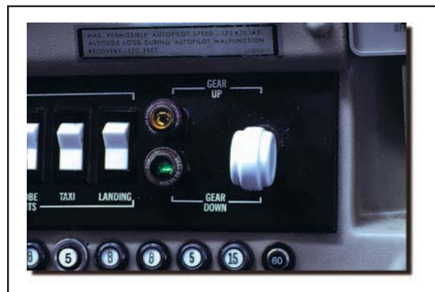
Figure 11-7. Typical landing gear switches and position indicators.
