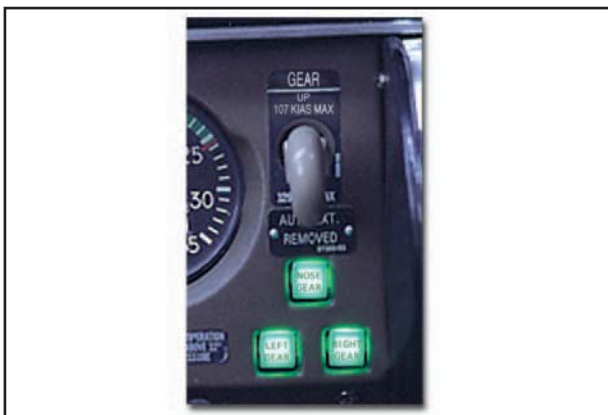
Figure 11-6. Typical landing gear switches and position indicators.
