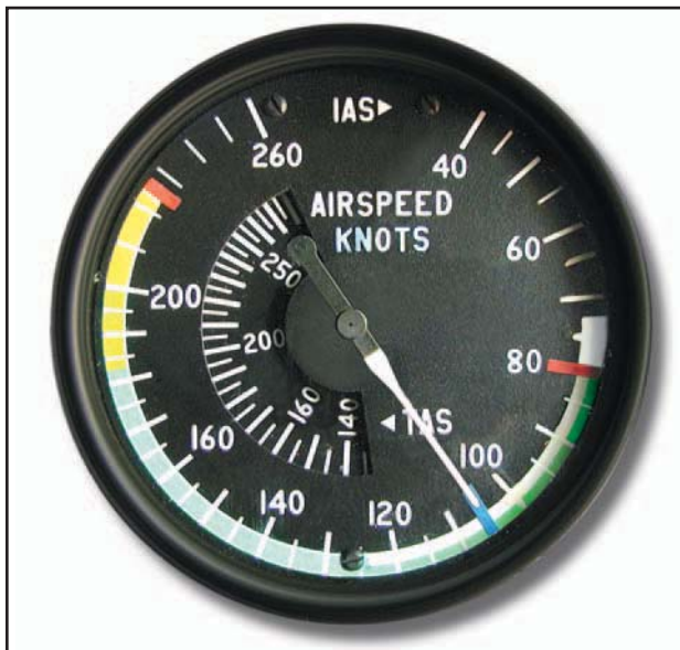
Figure 12-1. Airspeed indicator markings for a multiengine airplane.
