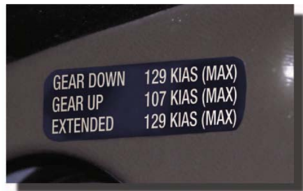
Figure 11-11. Placarded gear speeds in the cockpit.
