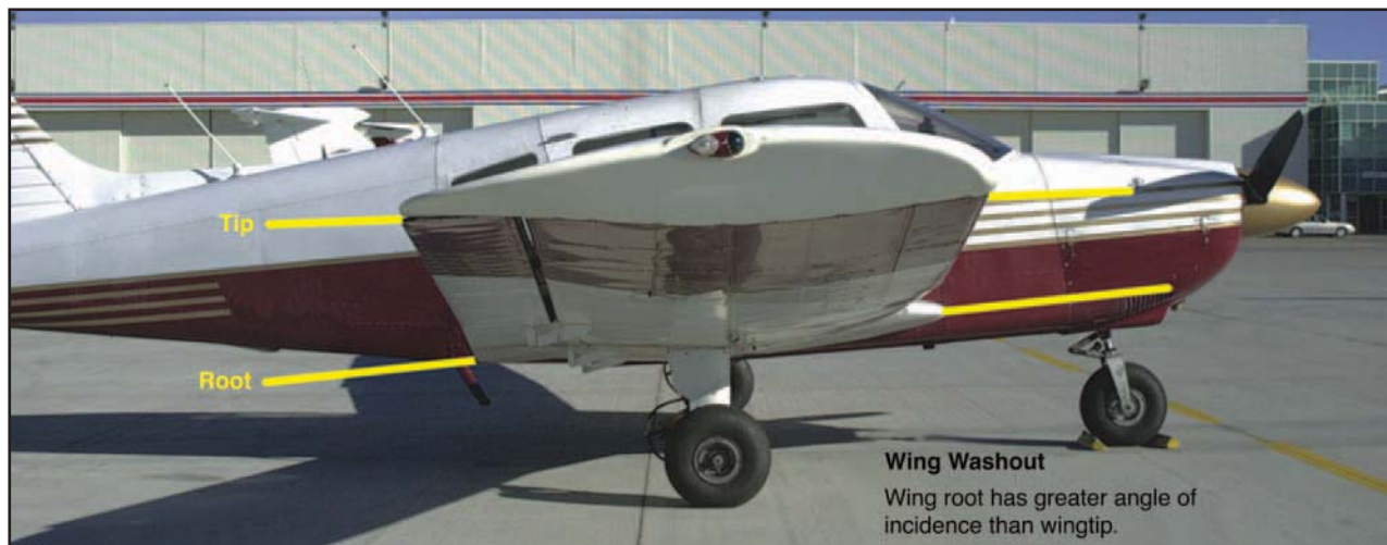
Figure 4-4. Wingtip washout.
