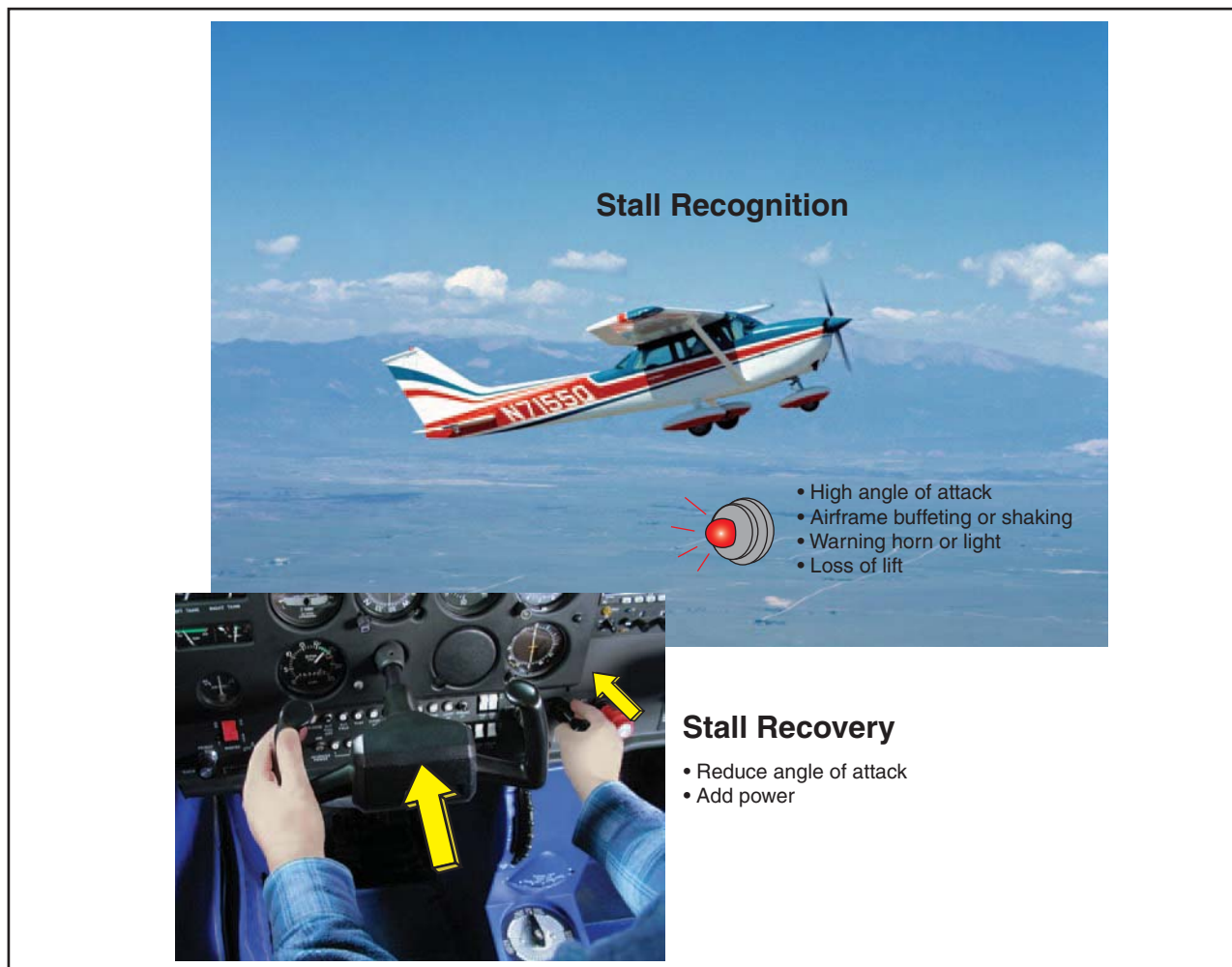
Figure 4-3. Stall recognition and recovery.
