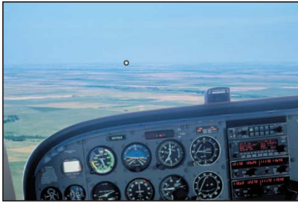
Figure 3-11. Visual reference for angle of bank.
