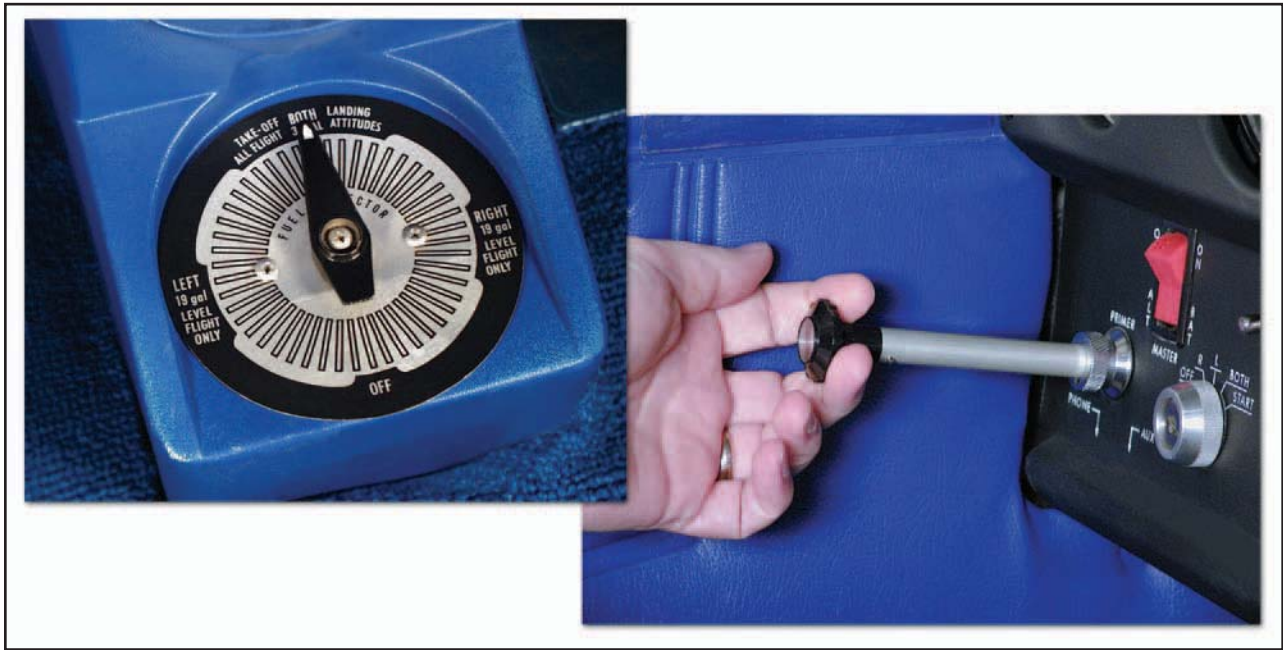
Figure 2-4. Fuel selector and primer.
