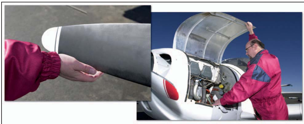
Figure 2-8. Check the propeller and inside the cowling.
