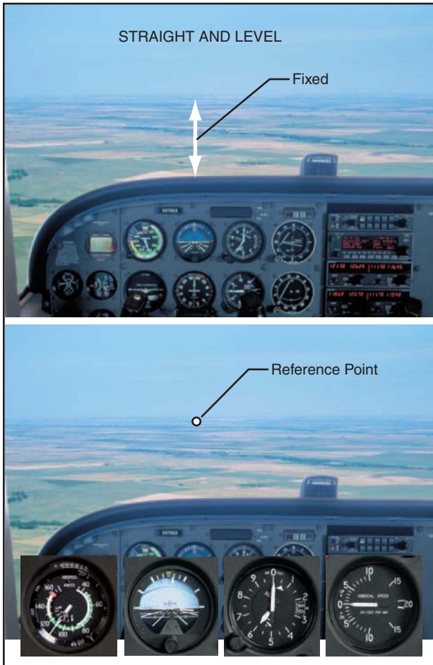
Figure 3-3. Nose reference for straight-and-level flight.
