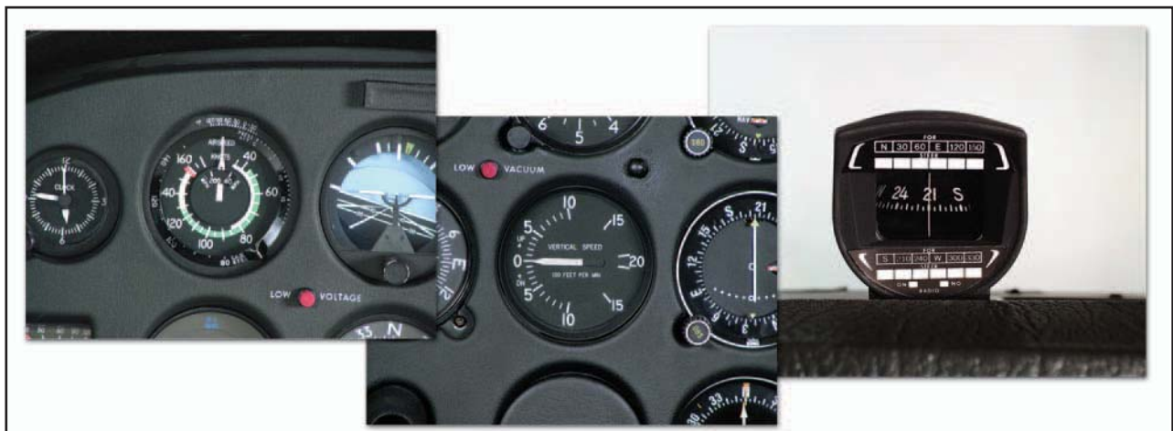
Figure 2-5. Airspeed indicator, VSI, and magnetic compass.
