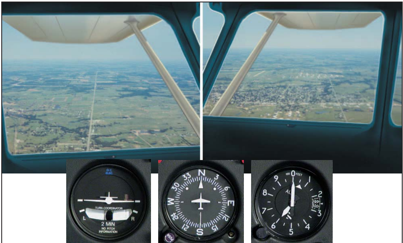
Figure 3-4. Wingtip reference for straight-and-level flight.
