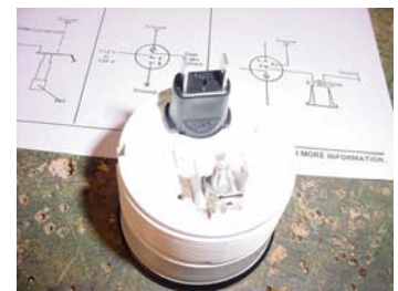
Back of gauge. The top two connectors are the light bulb (not required).
