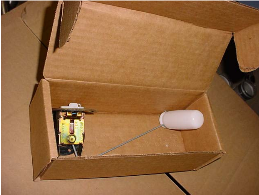
Float type fuel sender unit in supplier box Use VDO Fuel Level Gauge 73-10 Ohms P/N 301-029
