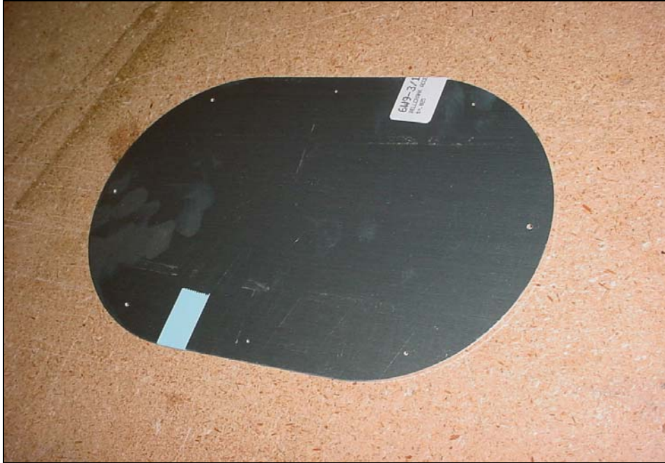
Aileron access cover 6W9-3
