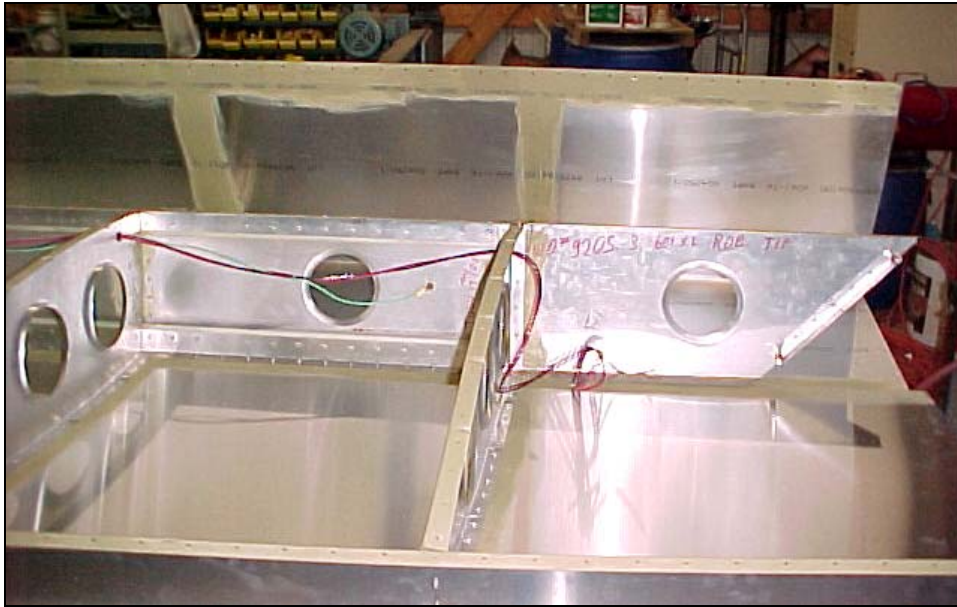
Alternative to using grommets; double tie wrap technique.
