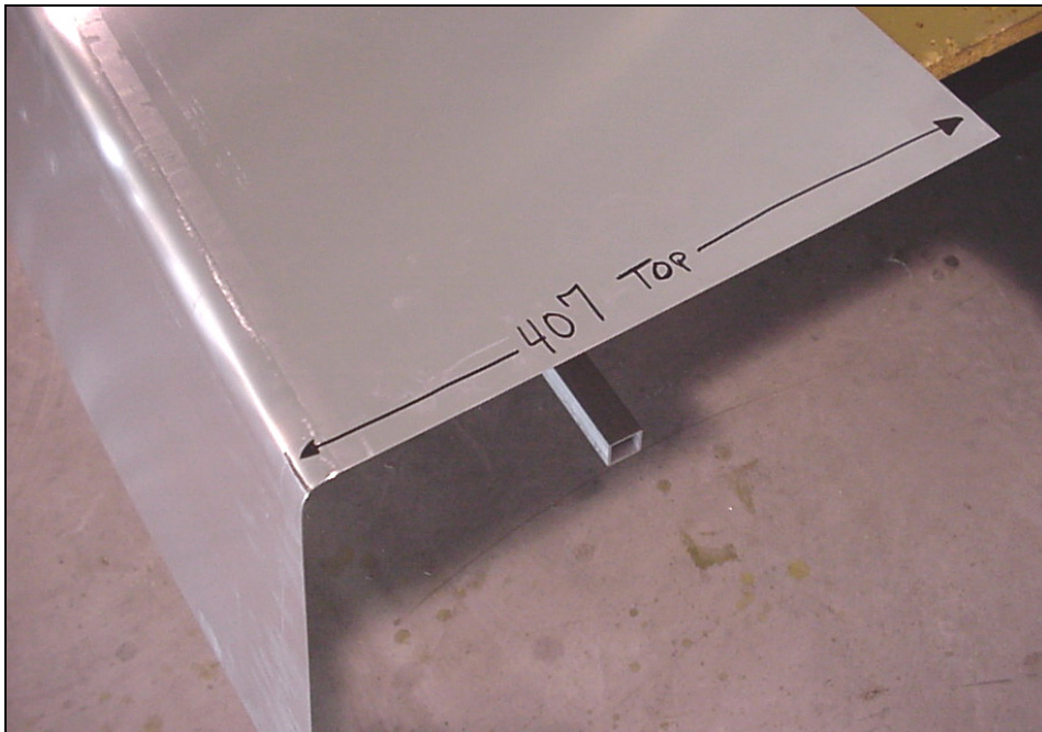
Clearly label the top and bottom side of the LE skin.
