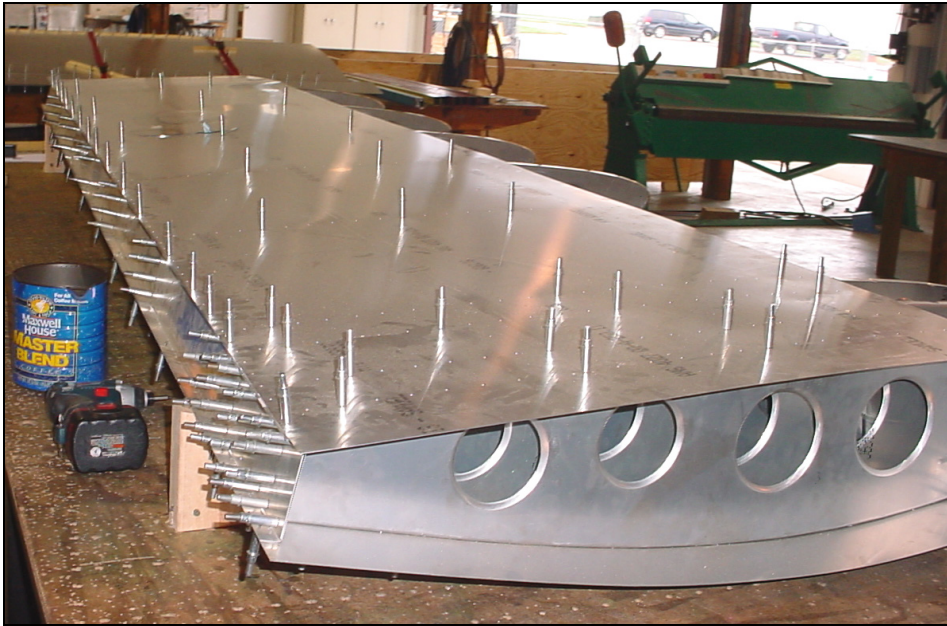
Support block under the rear channel.
