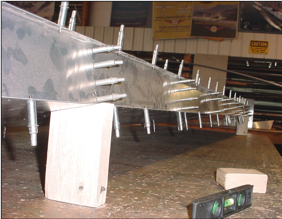
Check that the rear channel is level.
