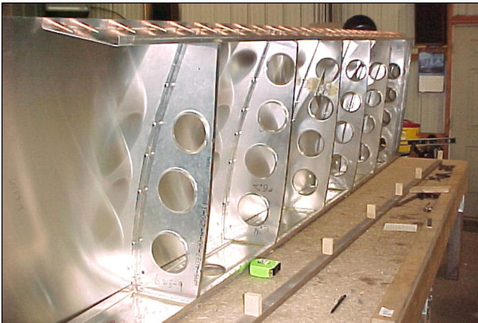
The tack rivets keep the wing skeleton from shifting as the wing is turned over.
