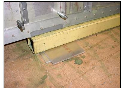
If necessary add shims between the workbench and the steel beam or spacer.
