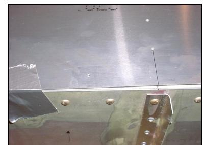
Use pieces of duct tape along the front edge of the skin to help hold the alignment.
