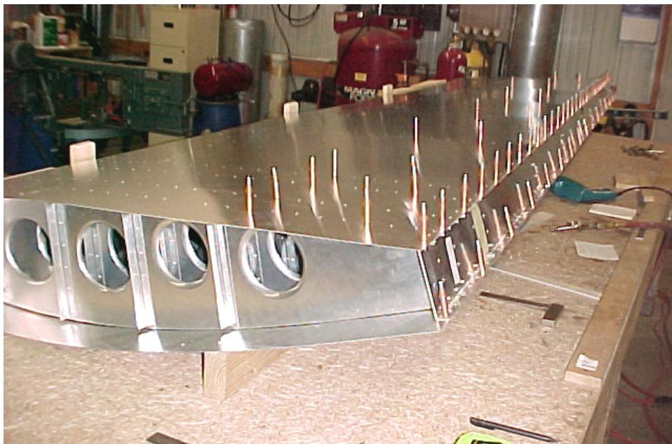
First drill through the rear channel. Drill from the back moving forwards.
