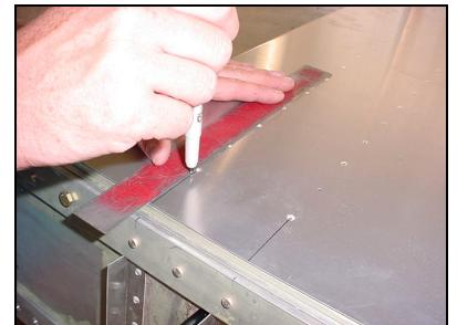
Also extend the rib rivet line to the front edge of the skin.
