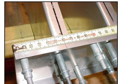
Mark the ribs station on the aft edge of the flange.
