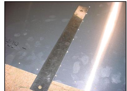
Mark the rib stations along the edge of the skin: use a straight edge to extend the center of the holes to the edge of the skin.
