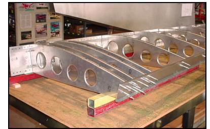
Check: Sight down the rear channel 6W7-1 and the spar, check that they are straight. The aft edge of the channel is the reference to position the Rear skins.
