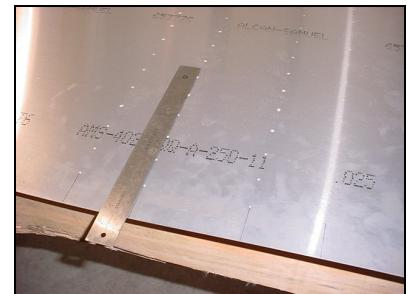
Also mark the rib stations along the front edge of the skin. Use a straight edge to extend the pre-drilled line to the edge of the skin.
