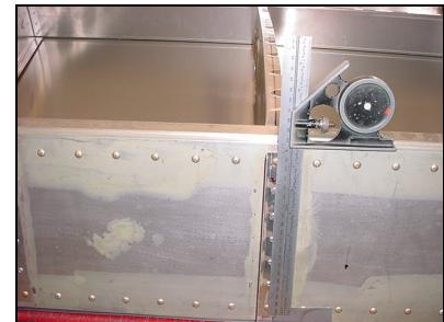
Note: the ribs stations shown on drawing 6-W-3 does not always correspond to the center line of the rib flange. Refer to drawing for the flange orientations.
