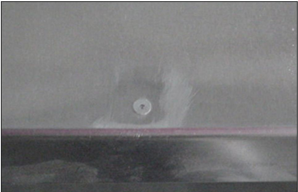
TACK RIVETS: they help keep the spar straight with the edge of the skin; they will also keep the ribs square as the wing is turned up side down to install the rear skin.
