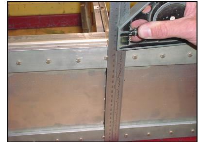
Mark the rib station along the top of the spar.
