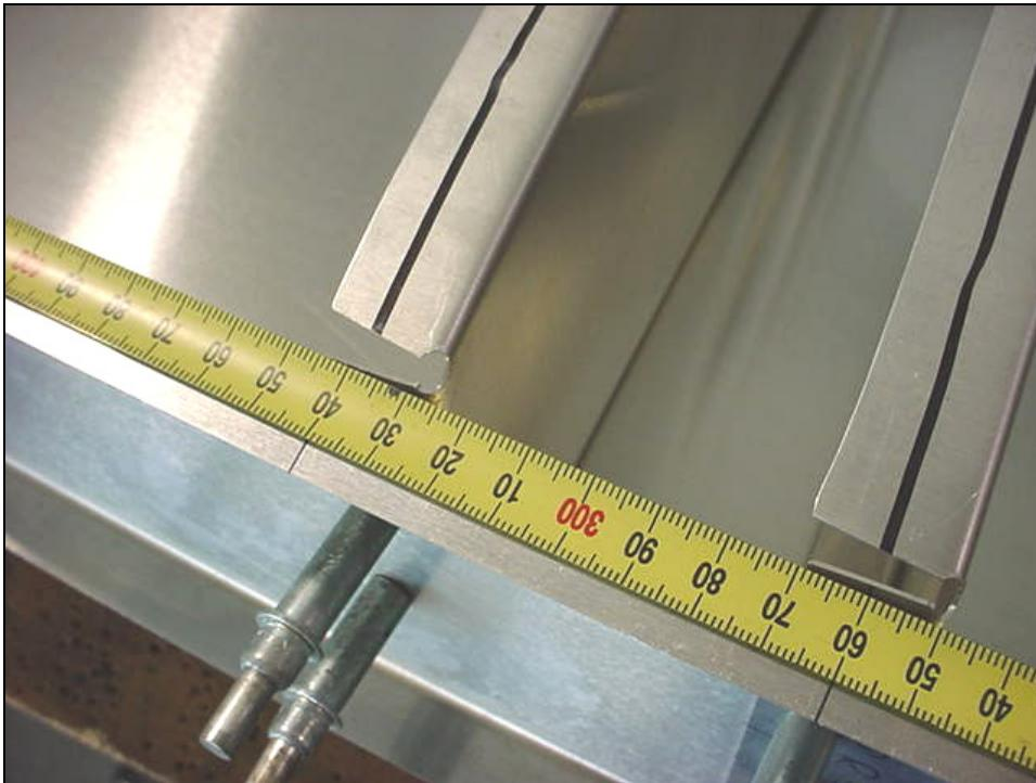
Layout & mark the rib stations along the aft edge of the rear channel, Ref 6-W-7
