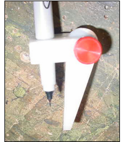
Edge marker block (adjustable) P/N 6352
