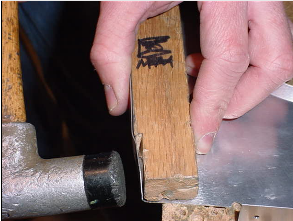
Joggling block: 3mm step by 25mm long
