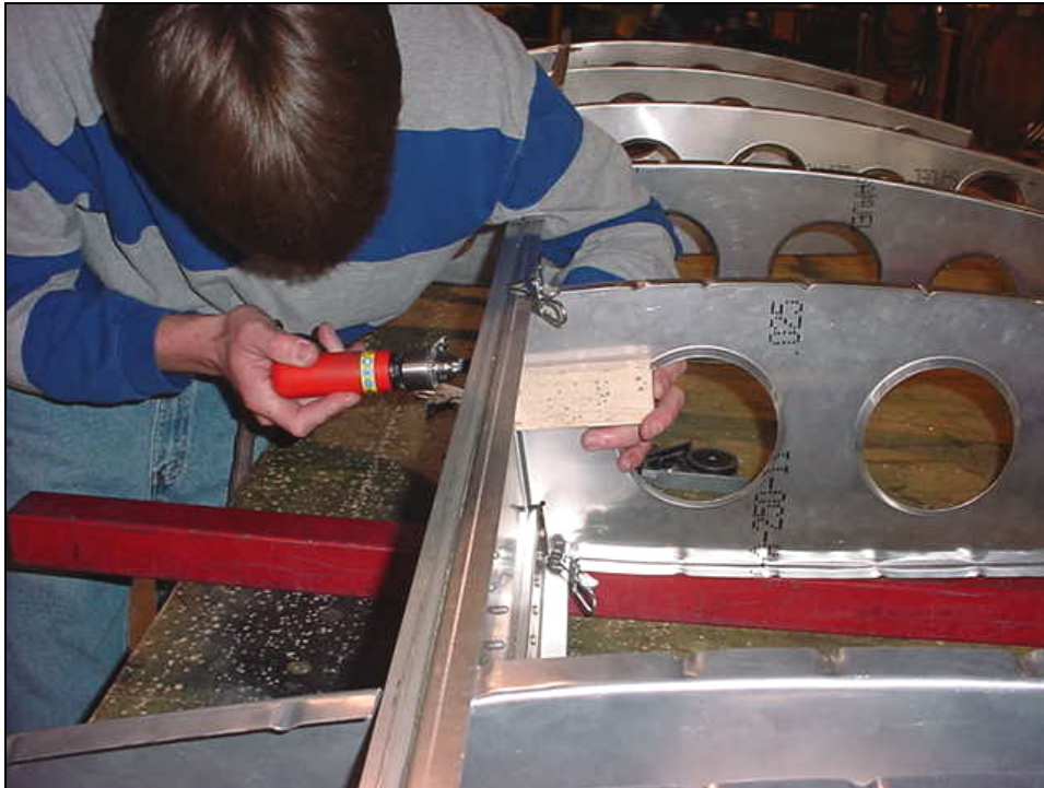
Backing block on the spar flange.
