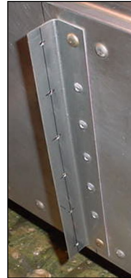
Layout the rivet pitch.
