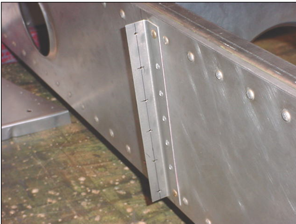
Layout the rivet line on the nose rib angles 6W3-9
