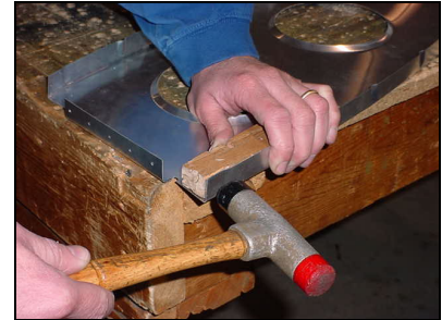
Joggling block: 3mm step by 25mm long
