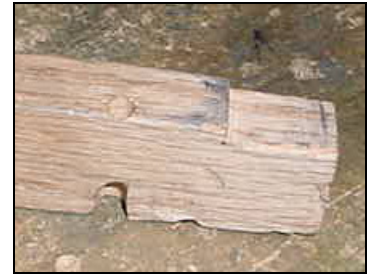
Joggling block: 3mm step by 25mm long
