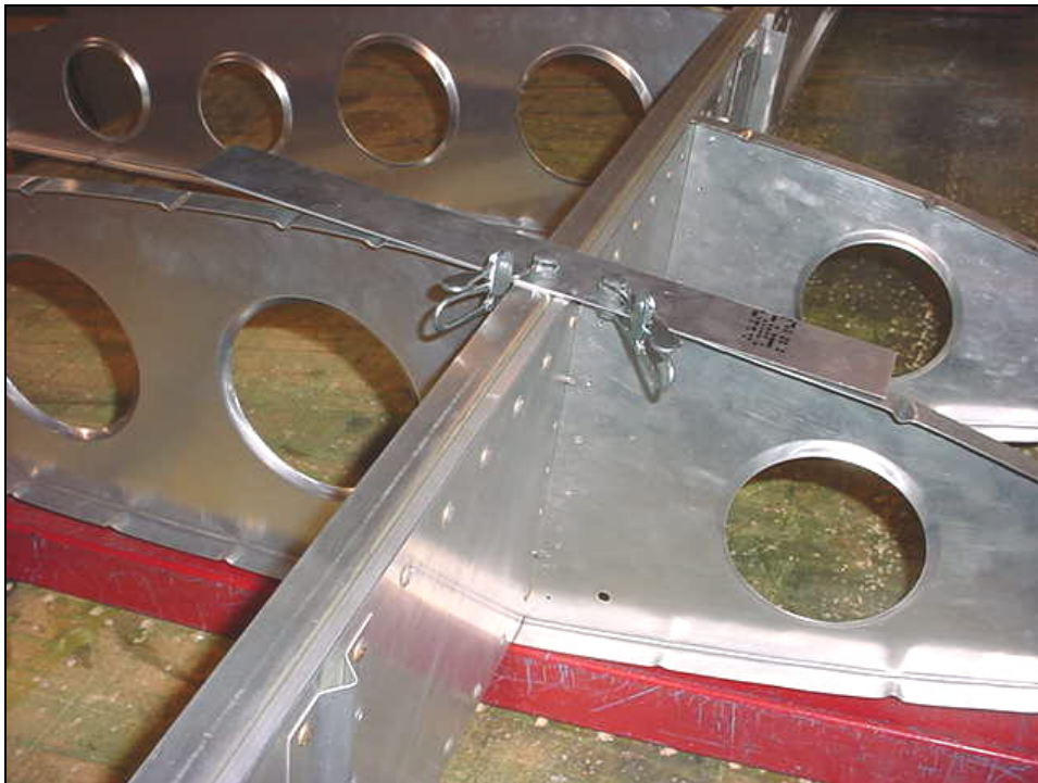
Check alignment, the height of the nose rib fits between the steel beam and the strip.
