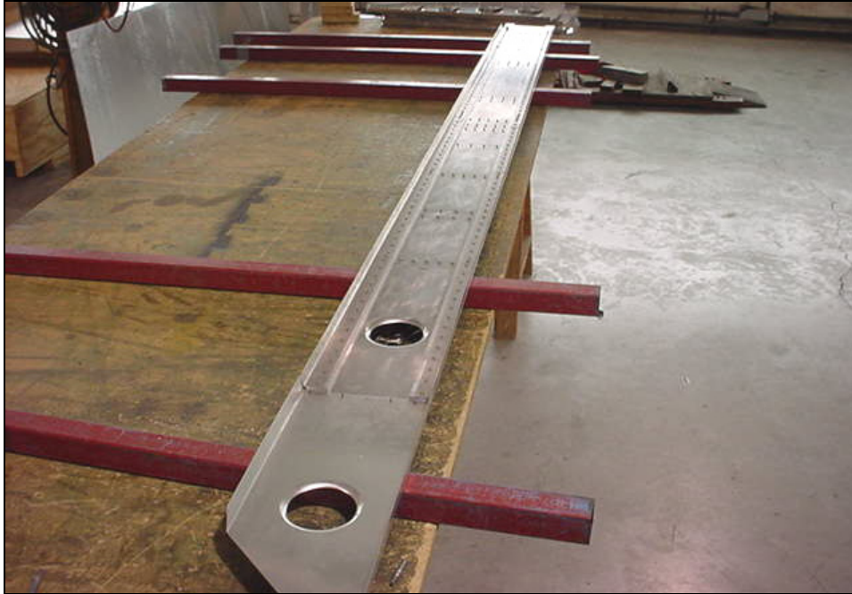
Steel beams (painted). Square 2"x2" length = 60" qty=6
