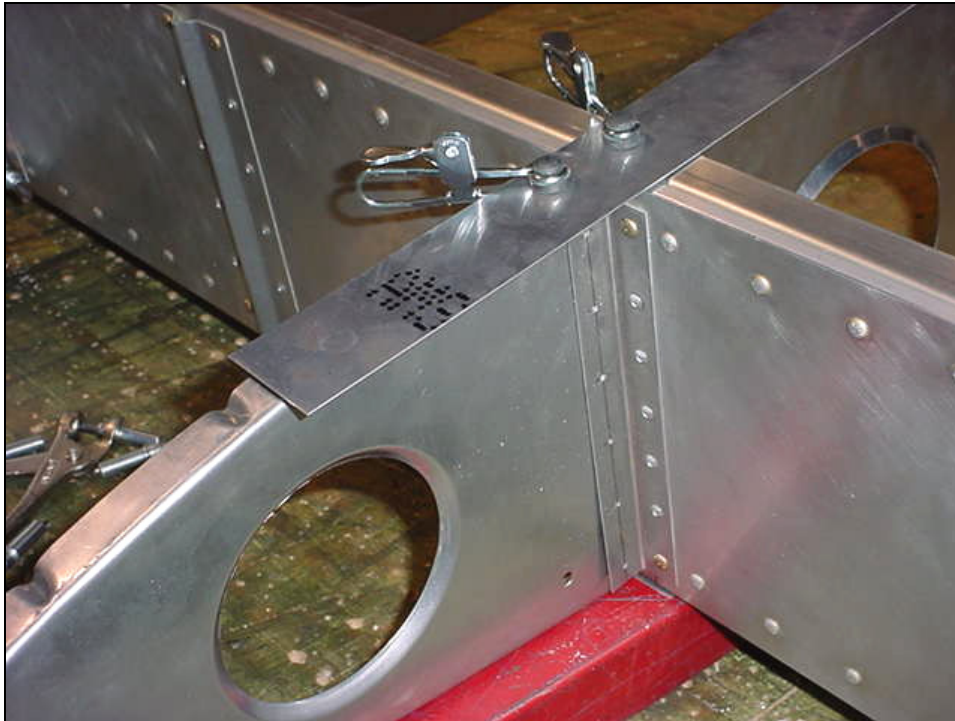
Position a nose rib and clamp the top flange of the rib to the strip.
