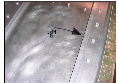
MARK: Identify the top side of the spar, and mark an arrow TOP (top spar cap angle 6W3-6 has the flange bend 90 degrees).
