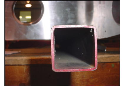
Steel beams (painted). Square 2"x2" length = 60" qty=6
