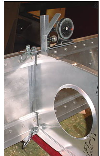
All the rear ribs are square to the top flange of the spar.
