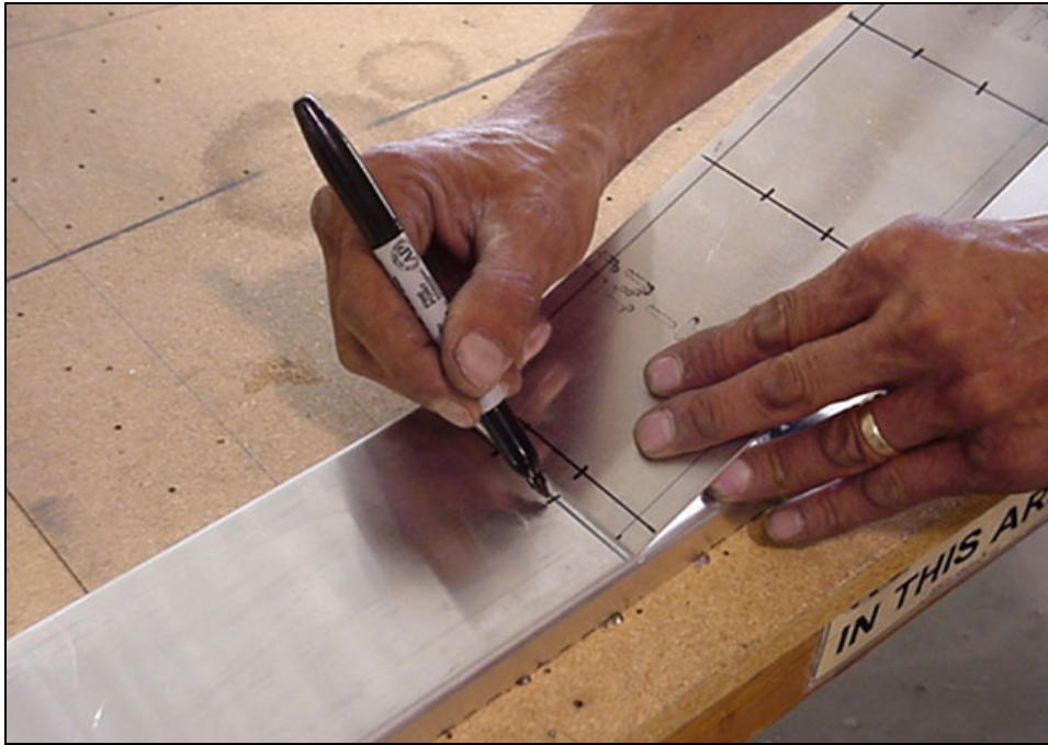
Using the Doubler to layout the rivet pitch
