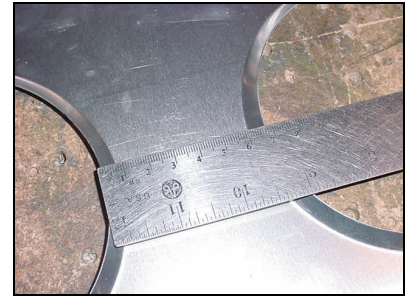
Layout the midpoint between the lightning holes.
