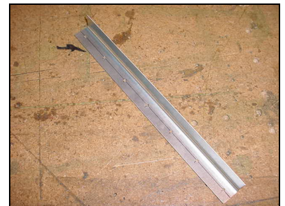
Pre-drill the L angles with #40 pilot holes.
