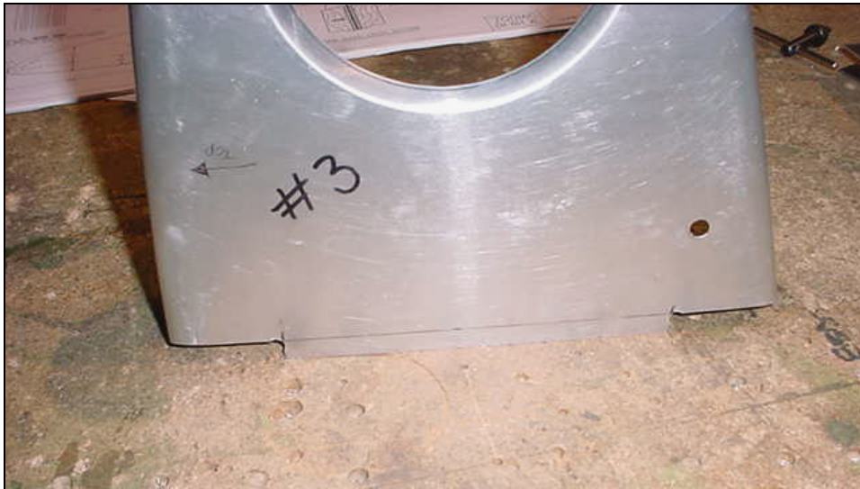
Nose Ribs 1, 2 and 3 See 6-W-7 for flange directions.
