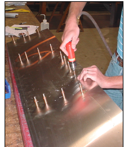
Drill the front flange.
