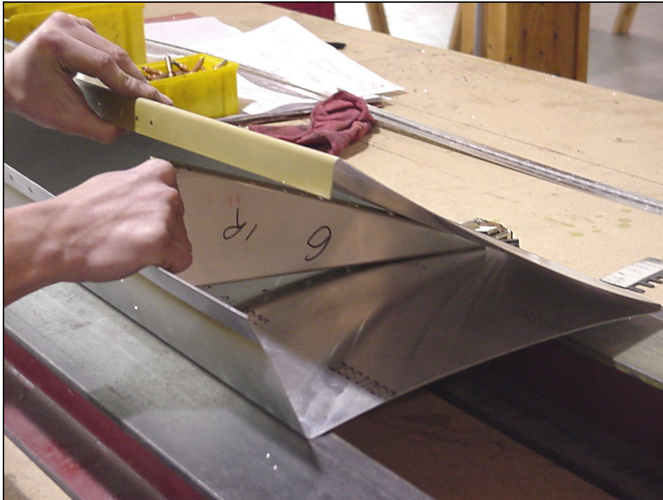
Position the ribs inside the flap skin.
