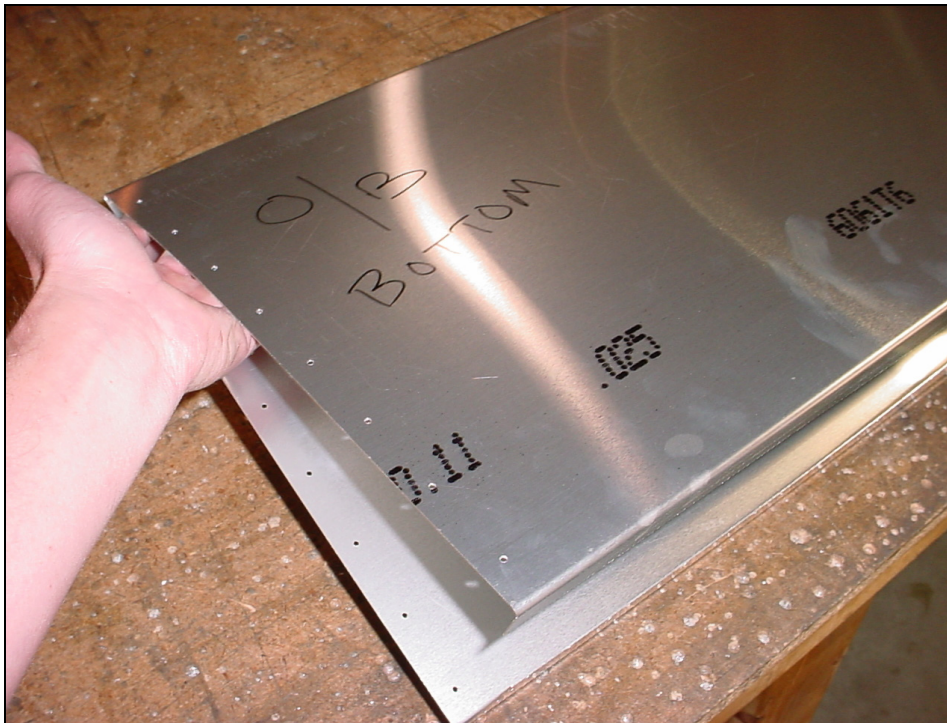
Pre-drilled holes in the skin.
