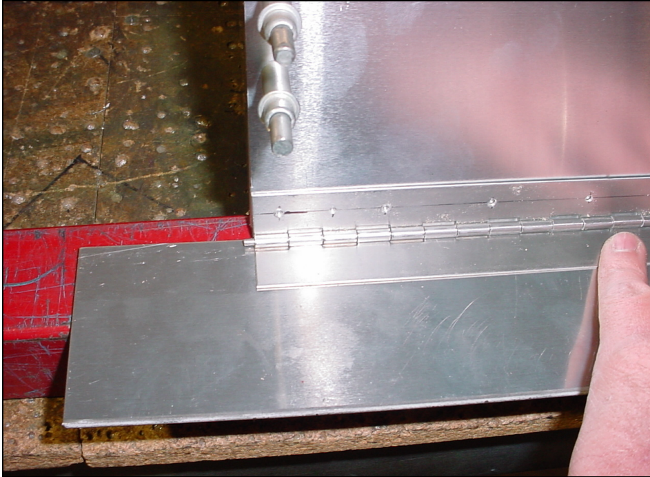
Rivet at the intersection of the rib station with the rivet line through the piano hinge.
