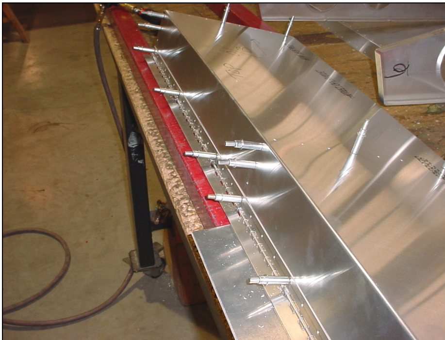
3mm offset from the bottom of the hinge to the bottom of the skin.
