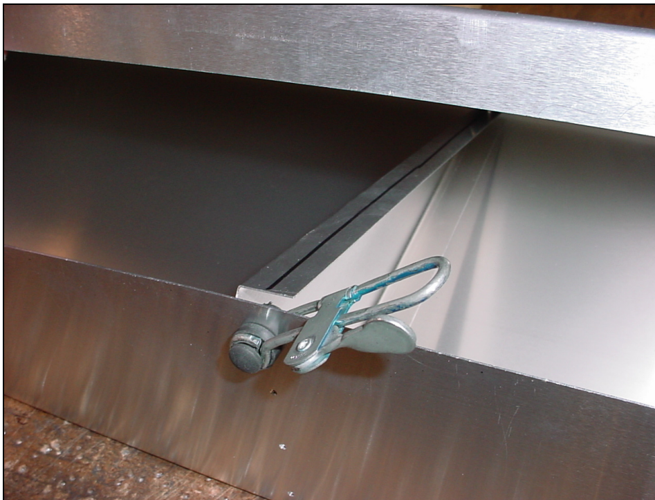
Clamp the front flange of the rib to the skin.
