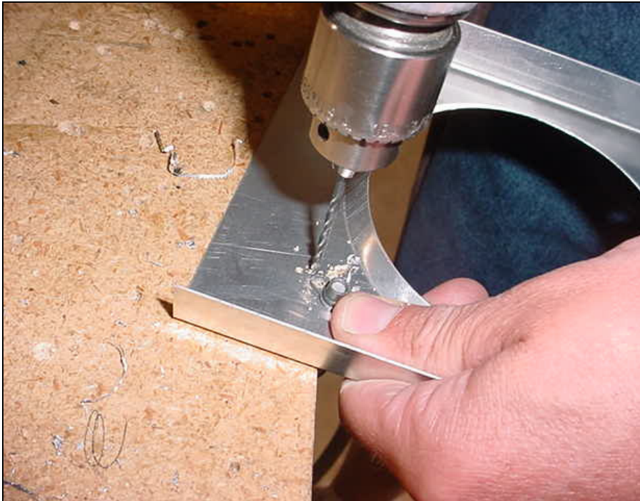
#20 drill bit. Back drill through the nutplate.
