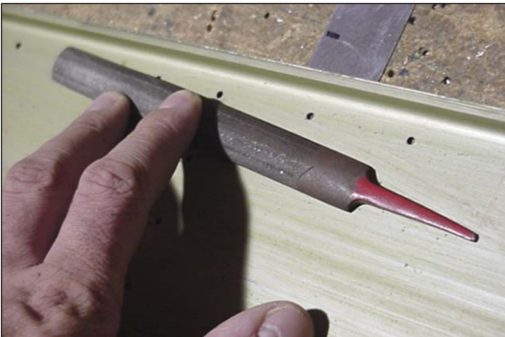
An alternative method is to use a large drill bit, and to give each hole a quarter turn. Remember to deburr both sides of every hole.
