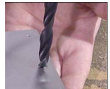
An alternative method is to use a large drill bit, and to give each hole a quarter turn. Remember to deburr both sides of every hole.
