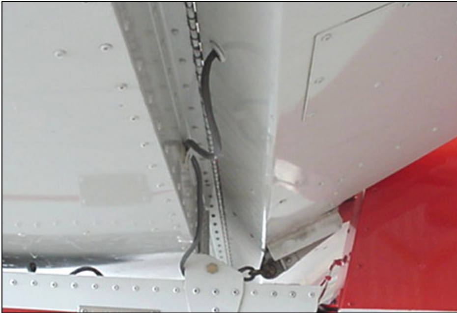
BELTON 5 WIRE The cable comes out the front of the elevator. Grommet located 30mm down from the top of the elevator. Grommet in the front of the elevator skin for the cable. AN931-4-7
