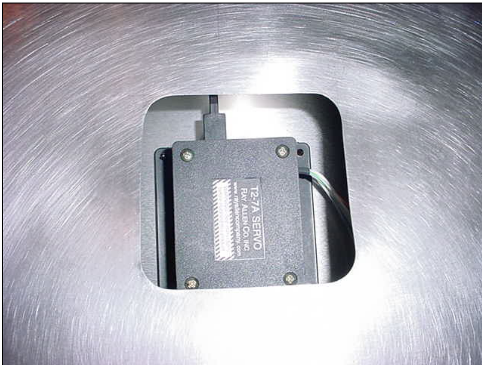
Detail of the servo clecoed to the underside of the topside of the elevator skin.
