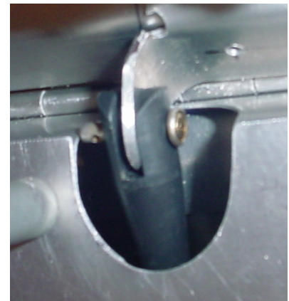
Install the Trim Motor arm assembly to the servo and to the Horn. The stainless steel threaded rod will have to be cut to length. Ref: bottom left diagram on 6-T-6.
