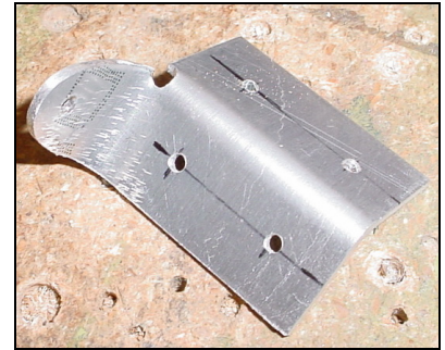
Pre-drill pilot holes.
