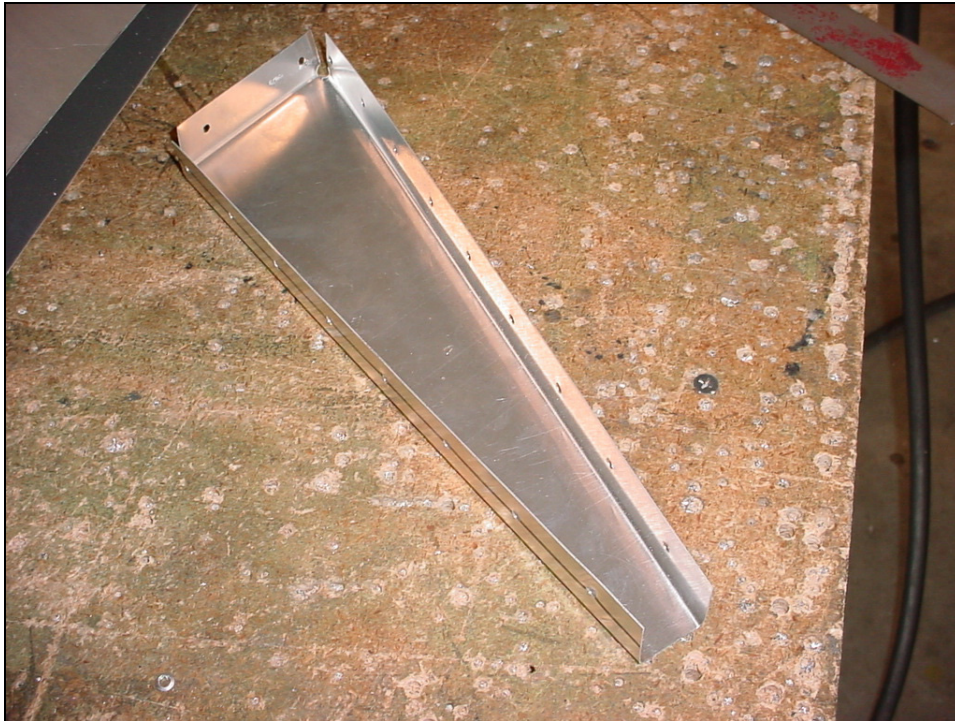
Middle rib 6T6-3, Ref. bottom middle diagram 6-T-6
