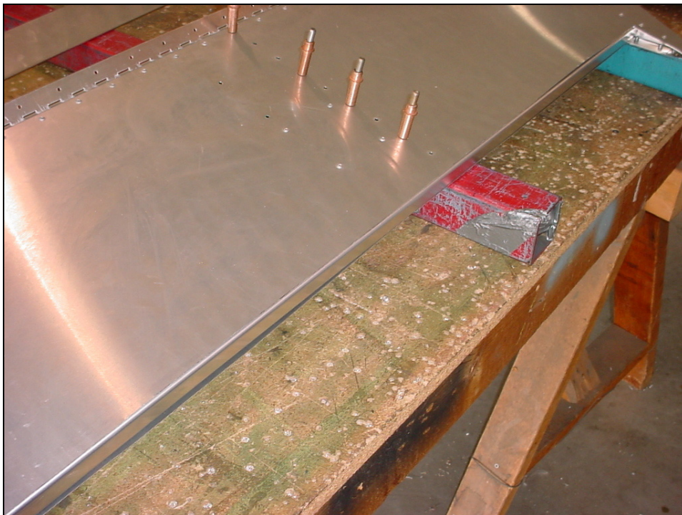
Install the channel with the web flush with the aft edge of the skin.
