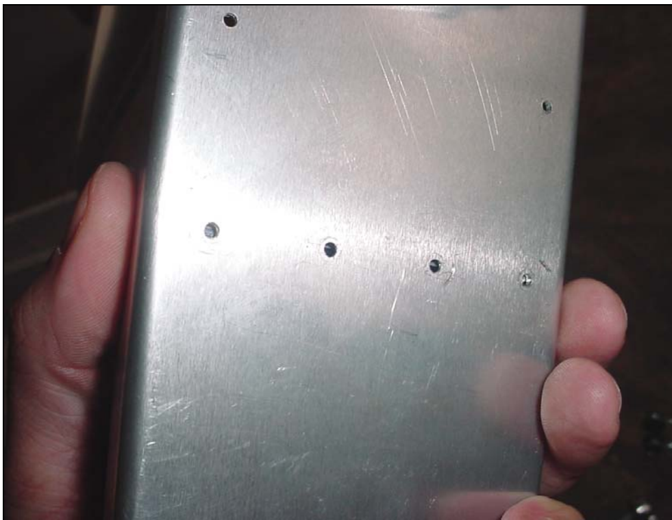
Adjust the position of the rib until the rivet line on the rib flange is visible through the pre-drilled holes in the spar.
