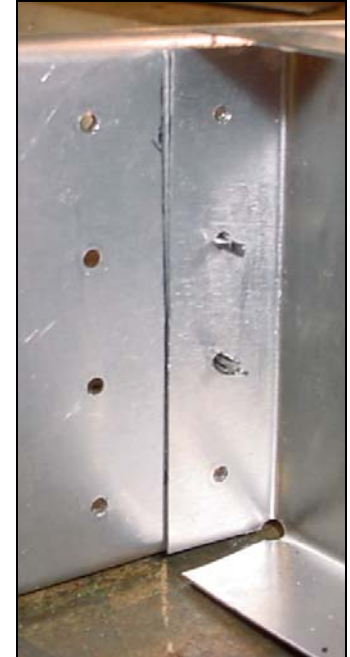
6T4-1 Drill and Cleco the nose rib to the spar.
