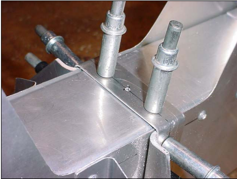
Detail of Bent Strip 6T3-8
