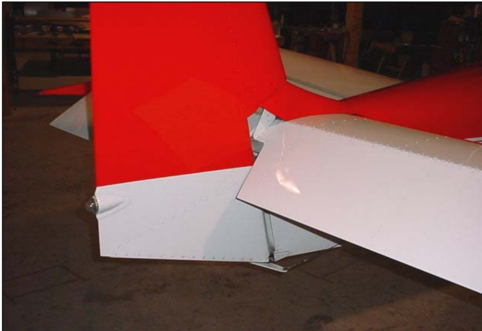
Gap between the skins around the rudder cutout is generally left open: with the rudder in place the gap is practically not visible!
