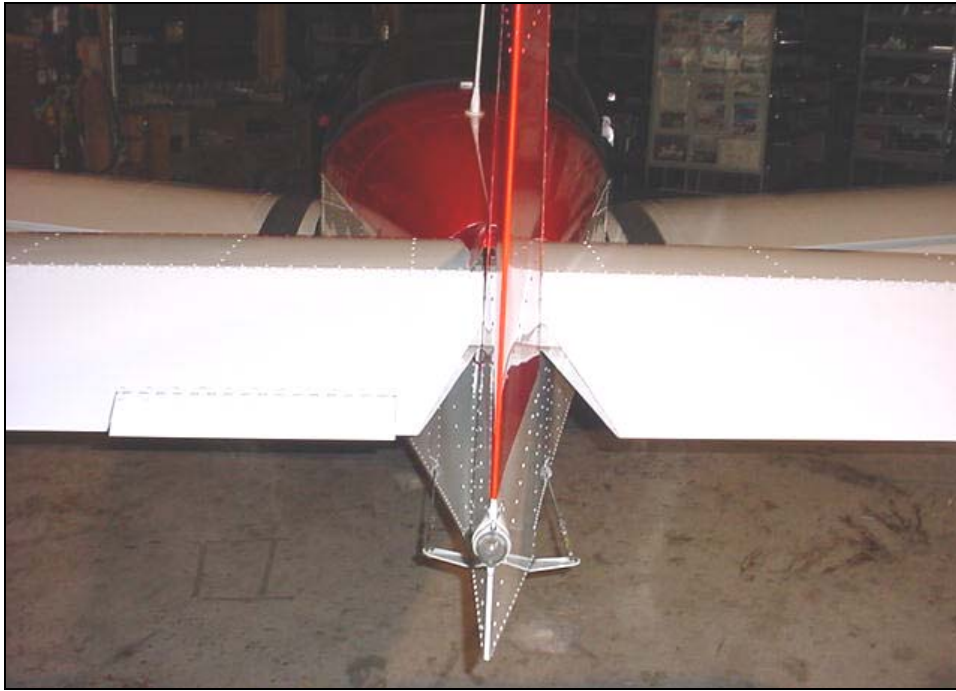
Rear view: elevator cutout to make room for the rudder deflections.
