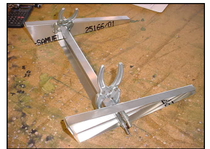
2 RIVETS A5 6T3-2 to "L" angle
