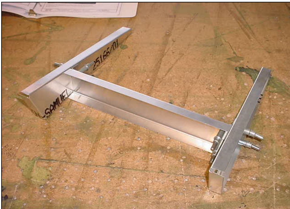
2 RIVETS A5 6T3-2 to "L" angle
