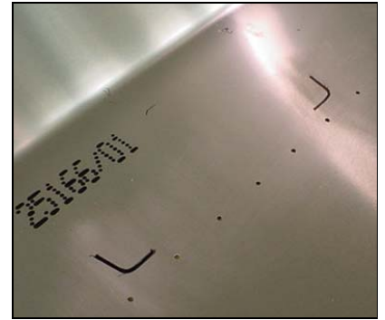
Detail: Cutouts for the Front Spar Attachment 6T2-1 (bottom side only).
