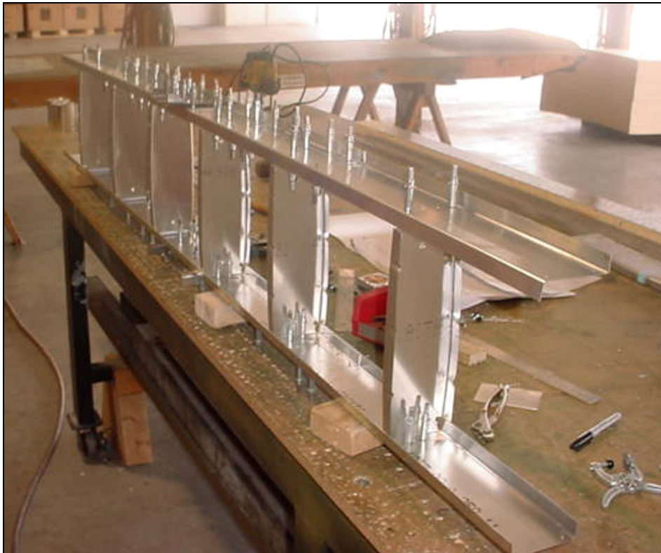
Line up the flange rivet line through the pre-drilled pilot holes in the spar.
