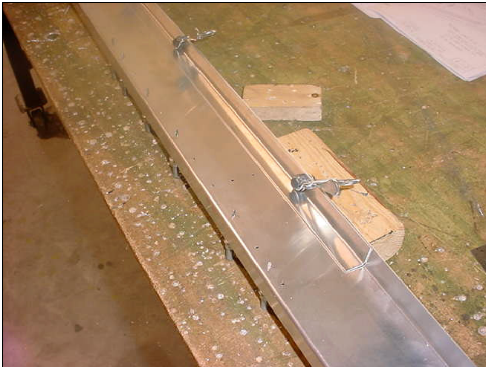
6T1-7HD clamped to the bottom flange.
