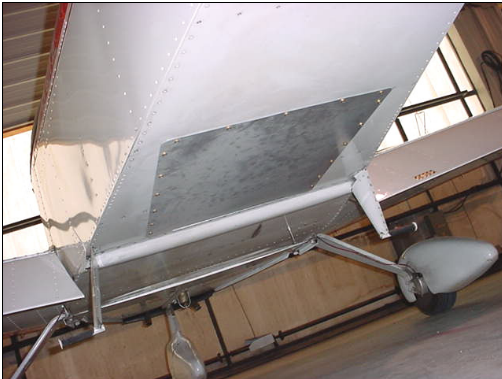
Access door located behind fuselage step fairing 6G3-5
