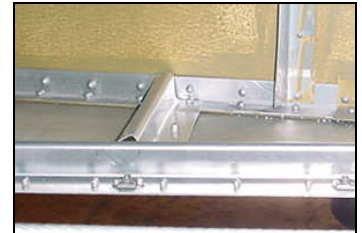
Short angle Cut and reinstall the short piece of L angle or Z angle between the longeron and the side Z angle
