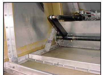
Access to flap control arm 6B19-2
