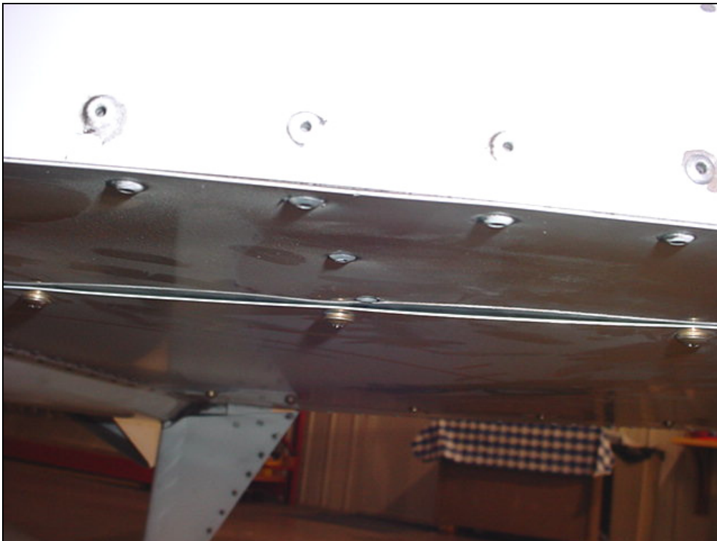
AN960-10 washer under screw.
