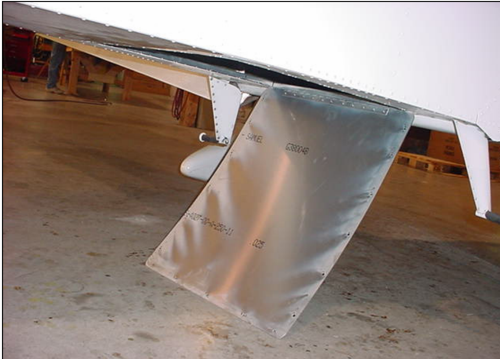
Access door hinged along front edge.
