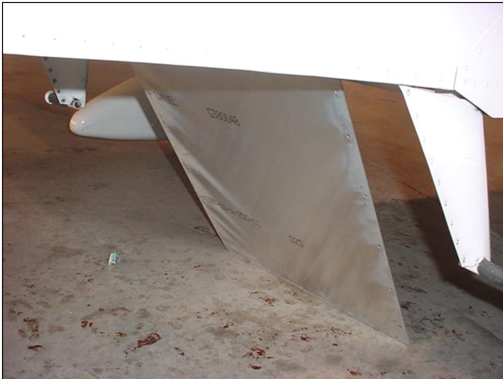
For better access inside the fuselage, the door can be flexed forward to stay out of the way.
