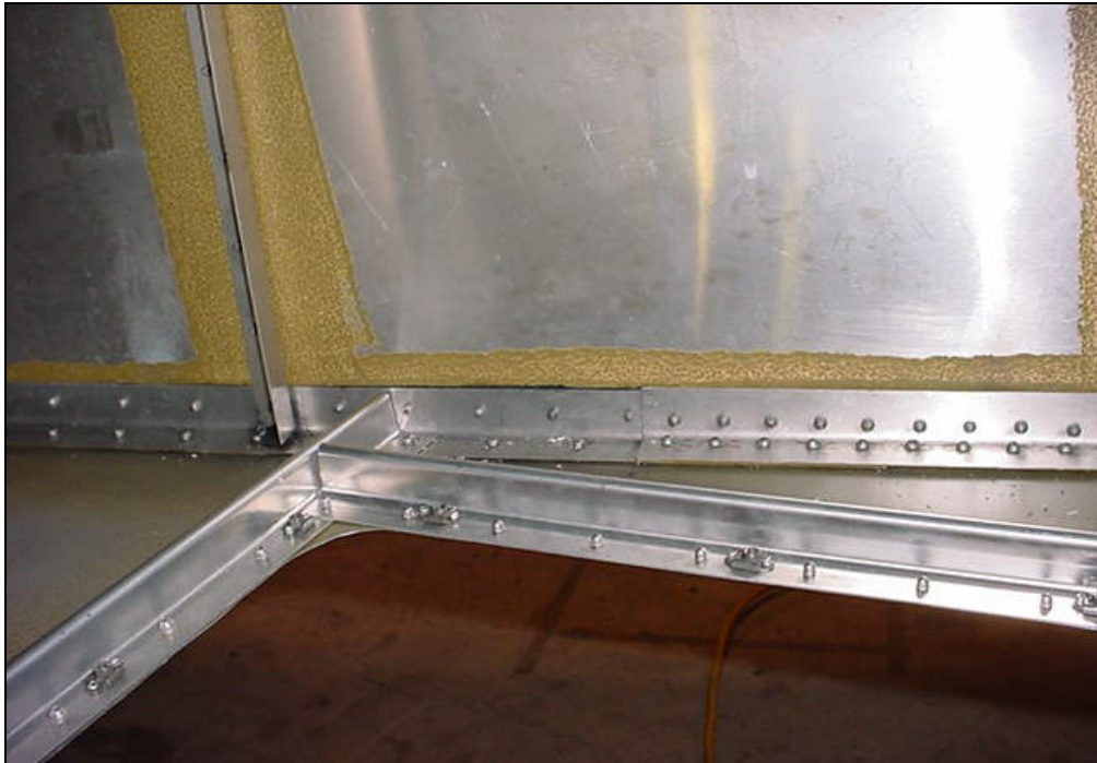
Short angle Cut and reinstall the short piece of L angle or Z angle between the longeron and the side Z angle
