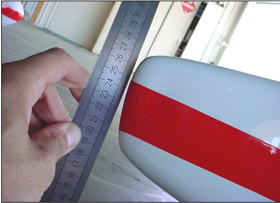
REAR: 250mm approximately (nose wheel fairing)
