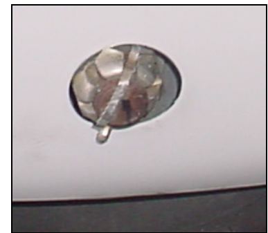
Use a step drill (uni-bit) to drill a round hole.
