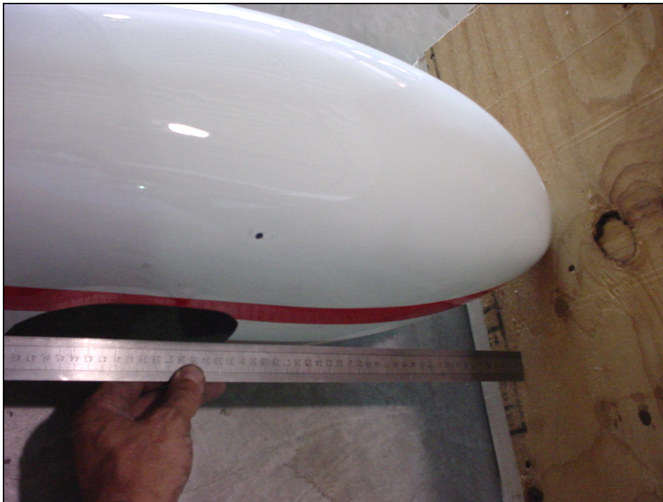
Layout the front and rear edge of the cutout for the gear and calipers.
