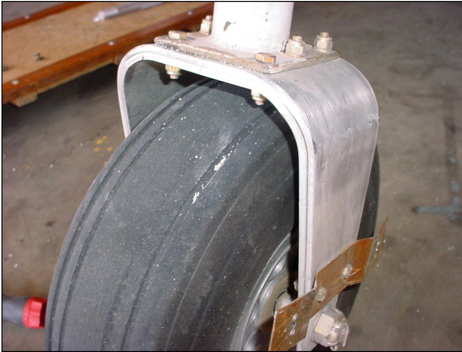
File a radius on the along the front edge of the fork doubler
