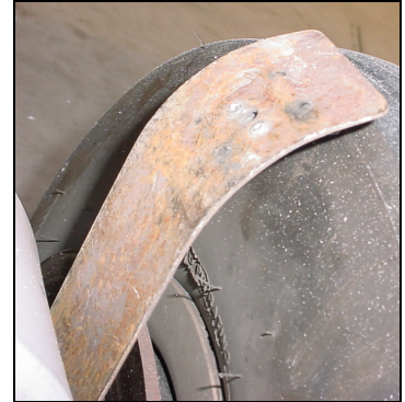
Install nutplate with 2 rivets A3
