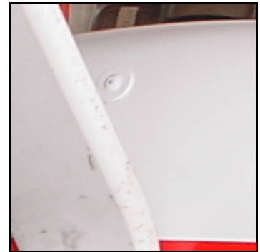
3 crews hold the wheel fairings in place. Photo of I/B screw
