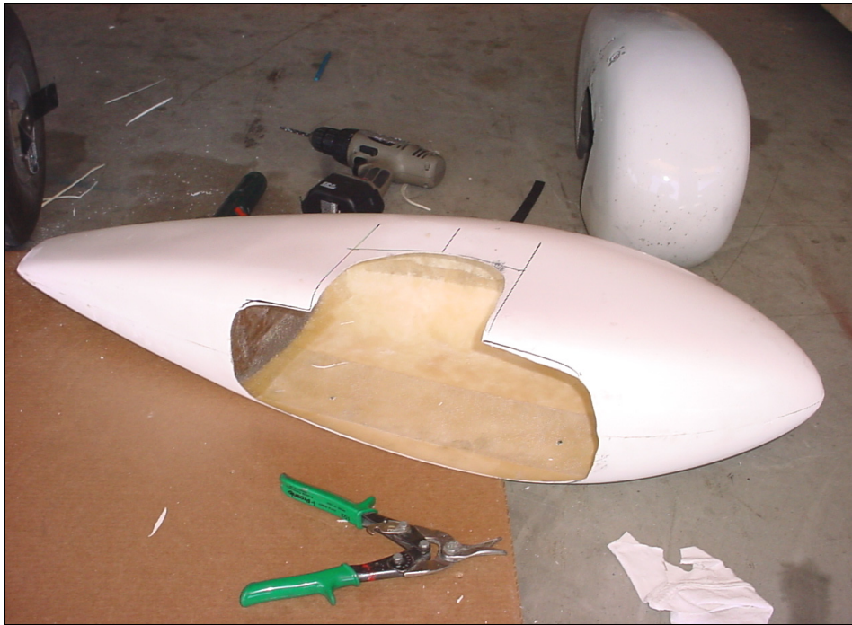
Radius the corners, see page 4 for installation on gear.
