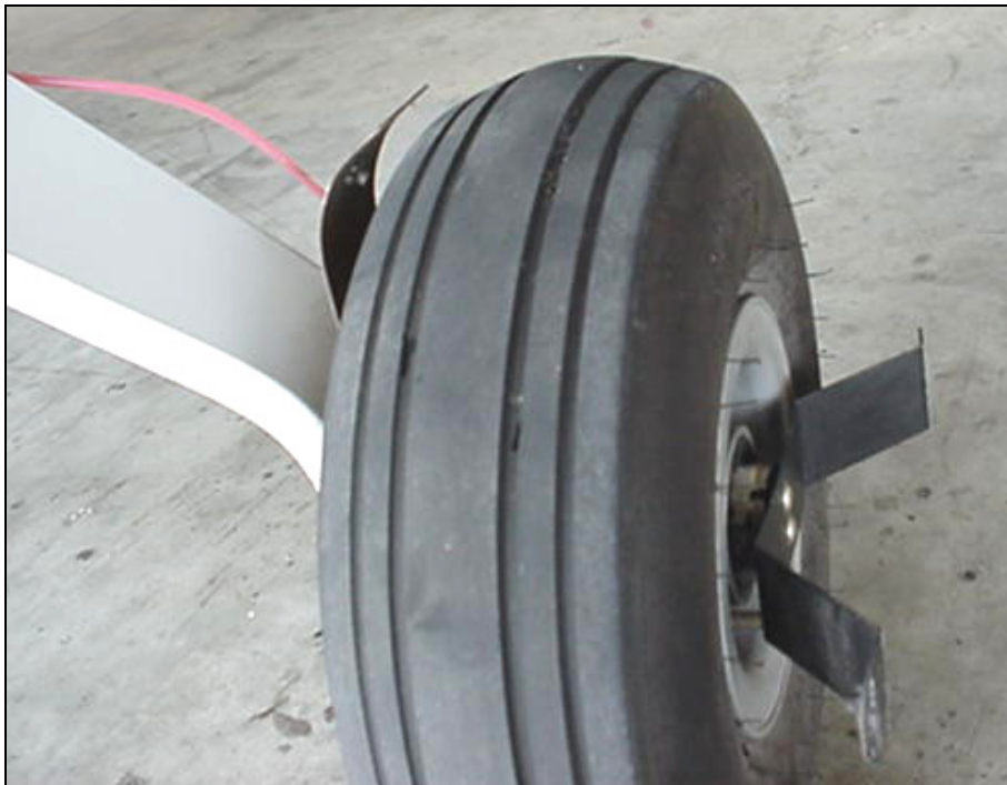
I/B and O/B wheel fairing attachment brackets
