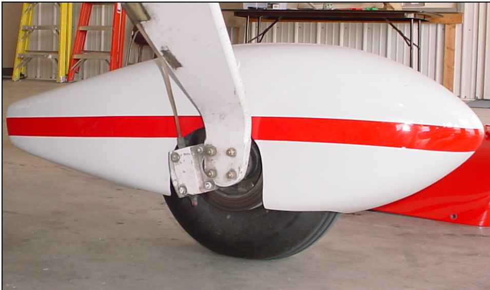
3 crews hold the wheel fairings in place. Photo of I/B screw
