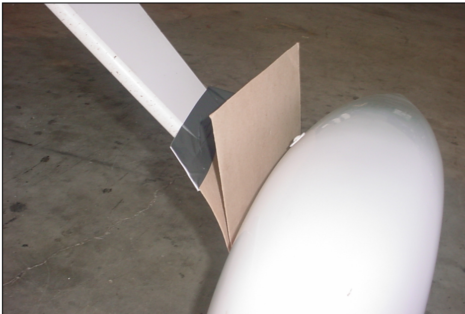
I/B Bracket 6-WFO-1-2 fits between the wheel axle and the outboard side of the rear. Bottom of bracket is installed even with the bottom of the gear.
