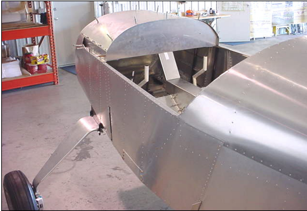
Gear is installed to the fuselage with the Main Gear Support 6G3-4
