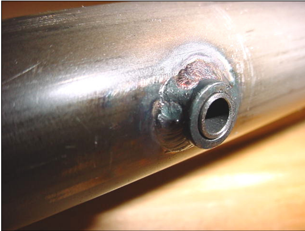
Detail of HT Bushing 6DS1-6 inside the 3/8" tube welded on the Torque tube 6DS1-5
