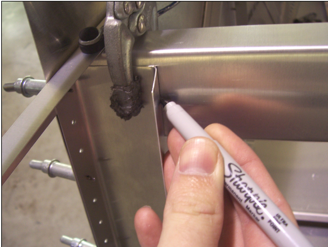
Mark the inboard edge and the top of the Upright Channel on the Upper Channel.
