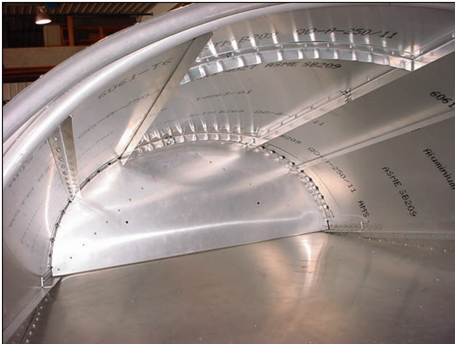
Crimped L angles between the two middle L angles for antenna reinforcement
