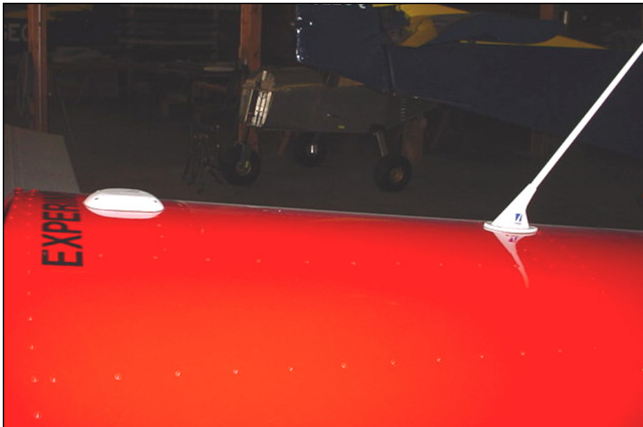
Com antenna in front of the baggage back bulkhead 6B12-2.
