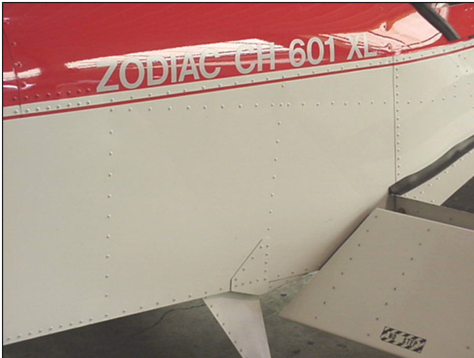
Detail of the longeron splice. Ref. 6-B-14
