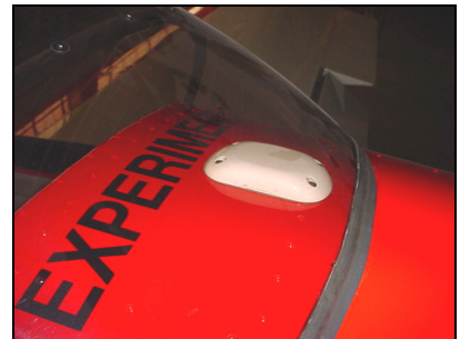
GPS Antenna fits nicely underneath the canopy.
