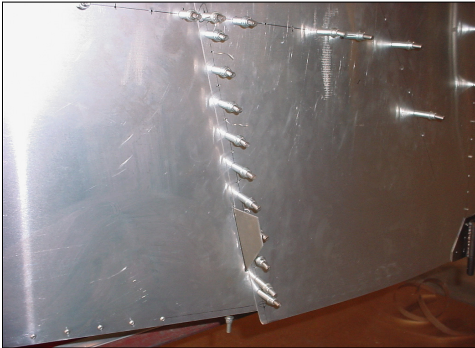
Drill and Cleco. A5 PITCH 20 Ref bottom middle diagram on drawing 6-B-21
