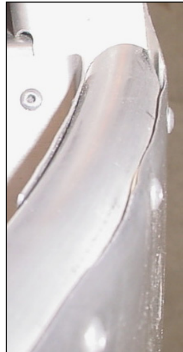
Top view of right side. It is normal to have a small amount of buckling between the rivets.
