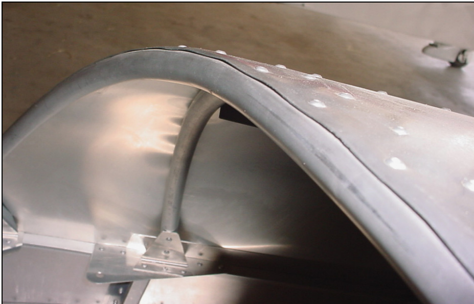
Wait to bevel the front edge until after the skin is riveted.
