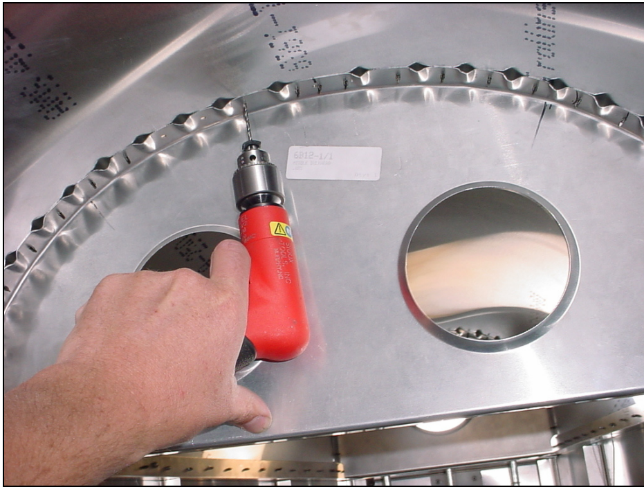
The middle bulkhead is back drilled by reaching in through the bottom fusealge access door 6-B-3
