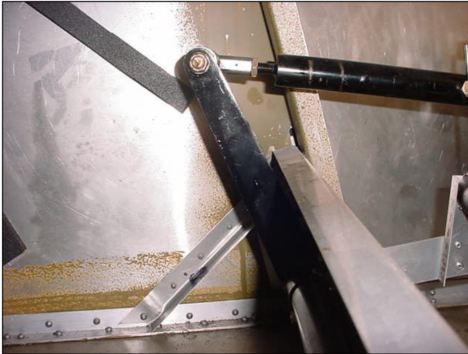
Detail of the flap control arm 6B19-3 in the flap up position. CHECK: There is some clearance between the front of the arm and the aft edge of the rear frame channel 6B5-2
