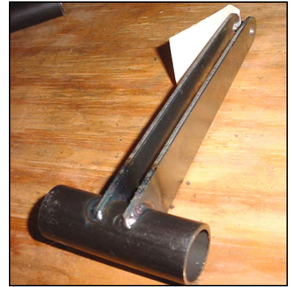
8B19-3 FLAP CONTROL ARM Welded assembly 1" inside diameter
