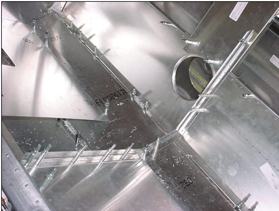
L angles along the front, bottom and back edge of the arm rest side 6B18-1.
