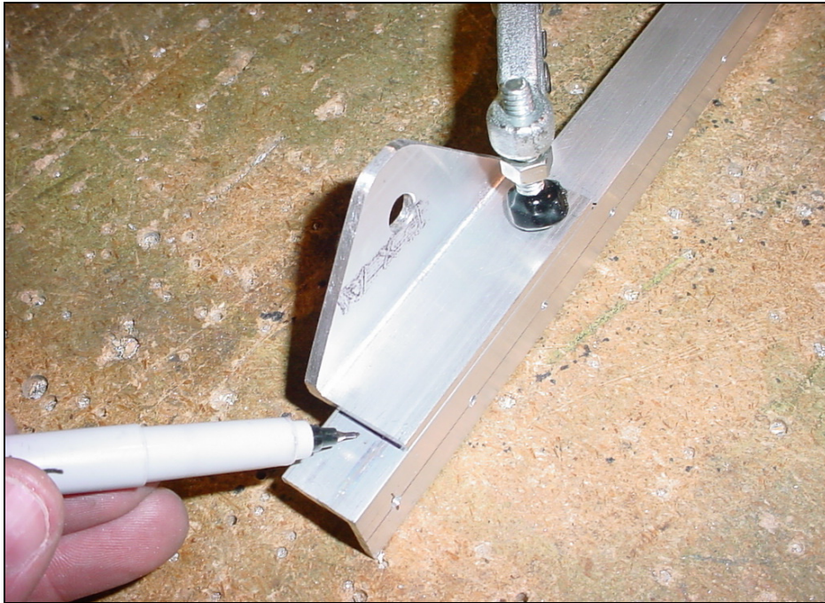
Remove the upright. Mark the top and bottom of the attachment on the extrusion.
