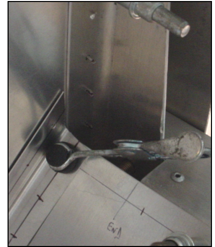
Clamp the L angle to the front seat panel 6B15-4
