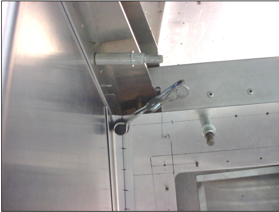
Clamp the L angle to the front seat panel 6B15-4
