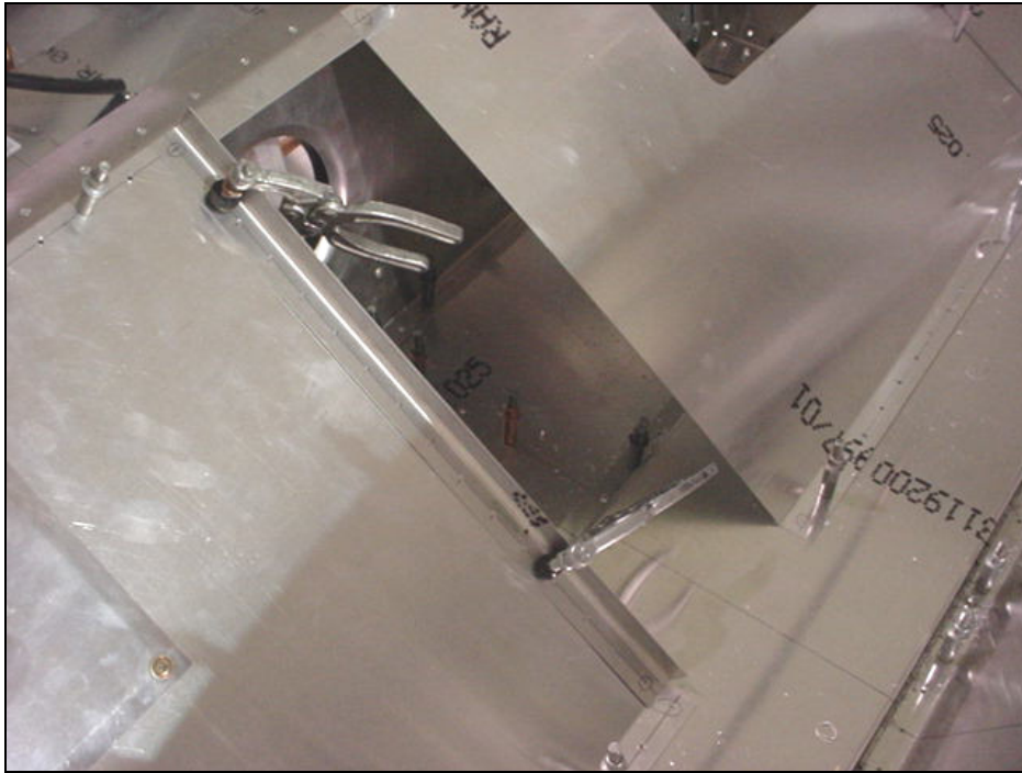
L angle along the I/B edge of the front seat panel 6B15-4.
