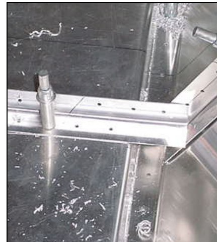
Detail of bottom aft overlap on top of the gear channel 6B5-5
