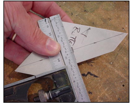
SEAT BELT ATTACHMENT DOUBLER PLATE 6B18-3
