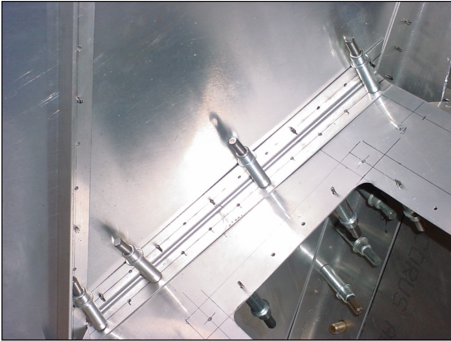
Another view of the L angle in the corner of the front seat panel 6B15-4 and the forward side skin 6B11-2
