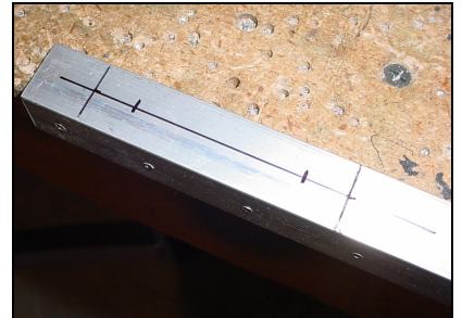
Clamp the seat belt attachment 50mm up from the top of the gear channel 6B8-5
