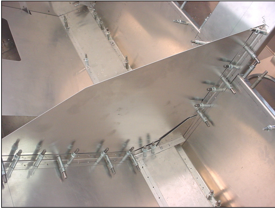
SEAT BELT ATTACHMENT DOUBLER PLATE 6B18-3
