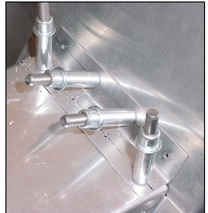
L angle in the corner of the arm rest cover 6B18-2 and the center seat back channel 6B16-2
