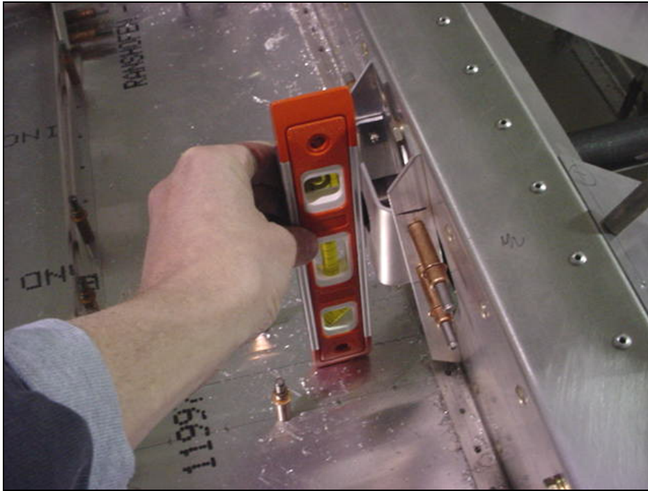
The bearing is square to the torque tube.
