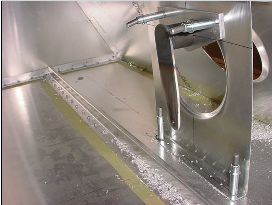
Rear view looking forwards. Drill and cleco the bottom flange of the rear torque tube bearing support 6B17-1 to the bottom skin 6B1-4
