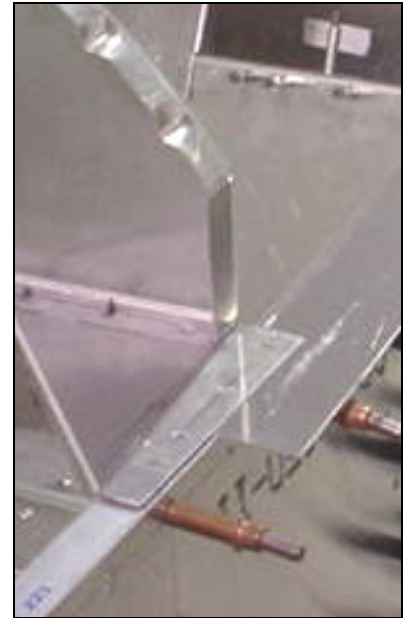
Front end, overlaps underneath panel gusset 6B12-5
