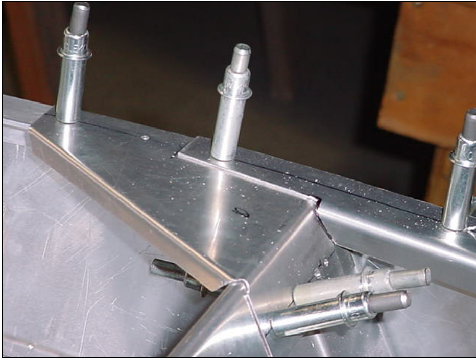
Detail of left side (rear) gusset 6B15-1
