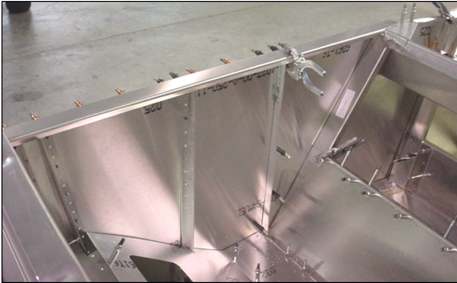
Trim parallel to the front flange of the baggage floor support 6B16-1.
