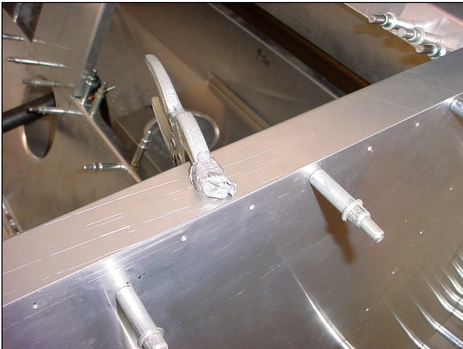
Position the front I/B flange of the doubler against the longeron, then adjust the doubler to bring the outer edge flush with the side of the fuselage and clamp in place.
