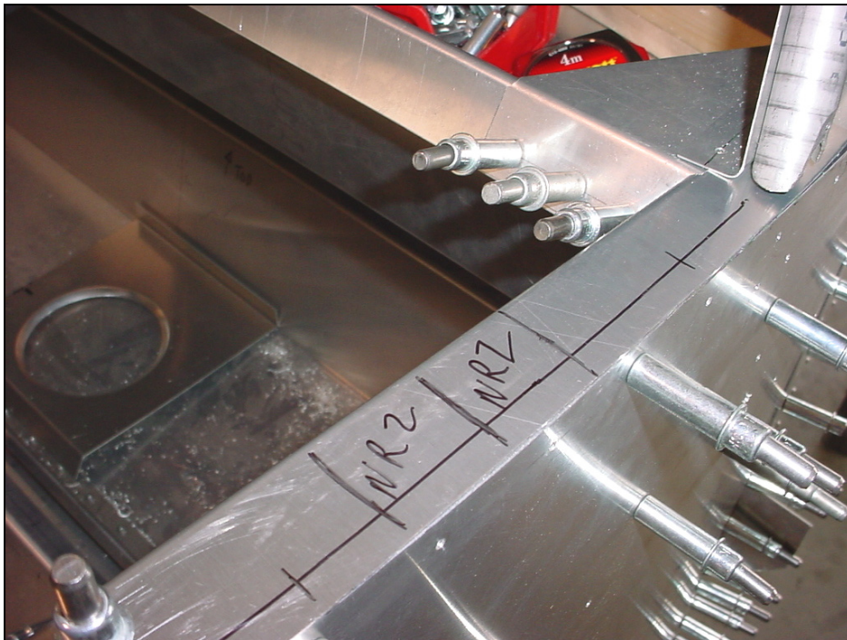
Locate the no rivet zone for the striker stud 6C2-1
