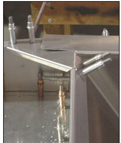
Trim back side flange to the same angle as the upper seat & baggage floor support 6B16-6
