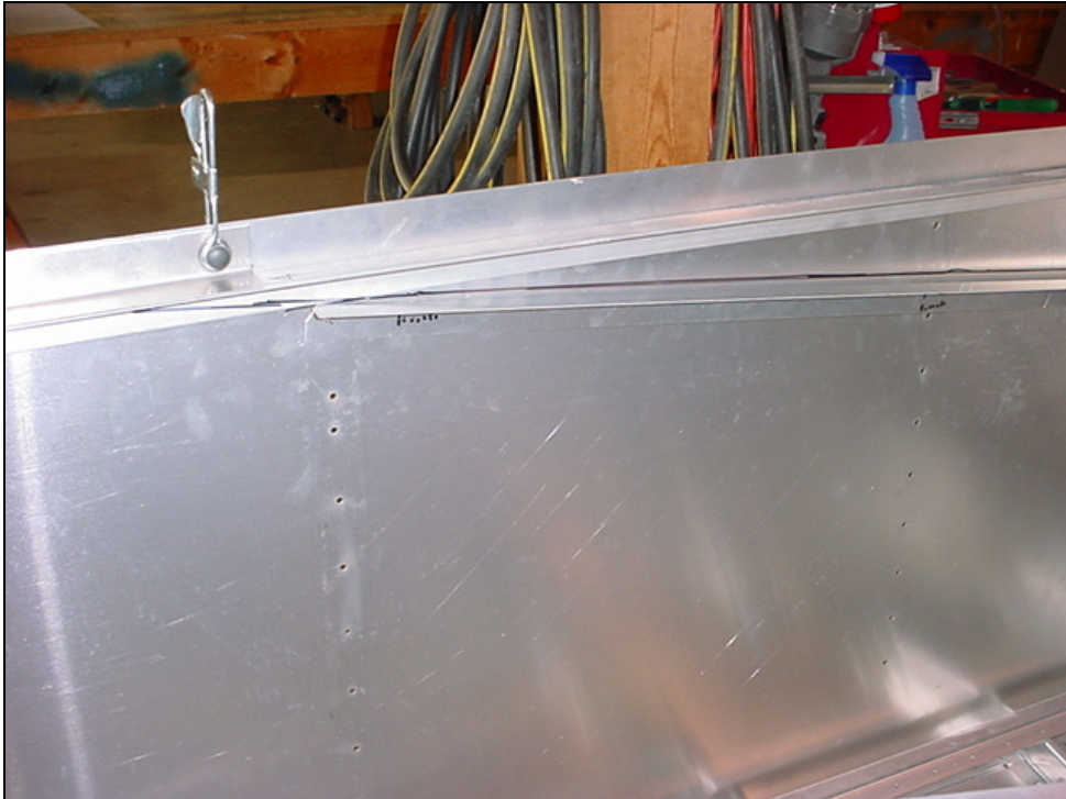
Looking at sloped rivet line in fuselage side skin 6B3-1 into corner L angle with the baggage floor 6B16-1
