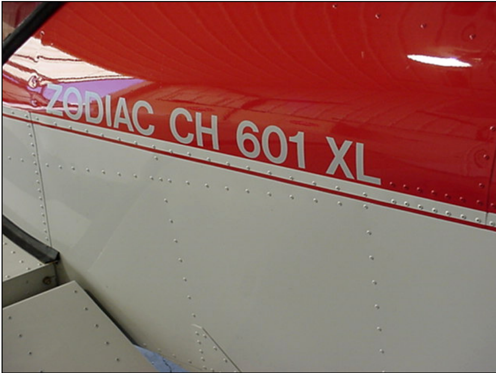
Looking at sloped rivet line in fuselage side skin 6B3-1 into corner L angle with the baggage floor 6B16-1
