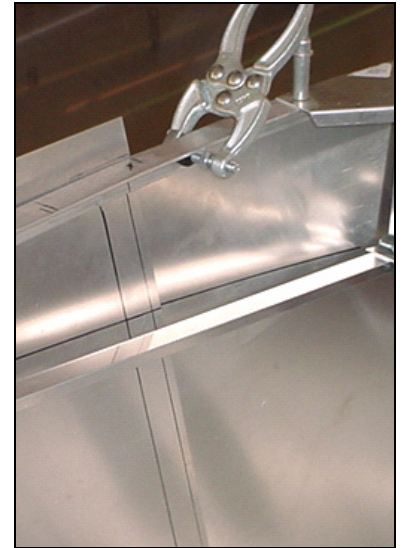
Note the gap between the fuselage side skin and the L angle.
