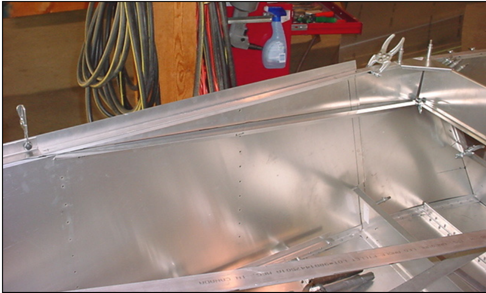
Clamp the L angle to the bottom flange of the floor support 6B16-6
