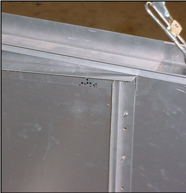
End of diagonal L angle even with aft edge of vertical L angle.
