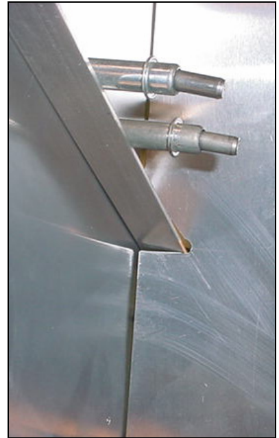
The cutout can be made L shaped as shown in this photo or triangular as shown on drawing 6-B-15
